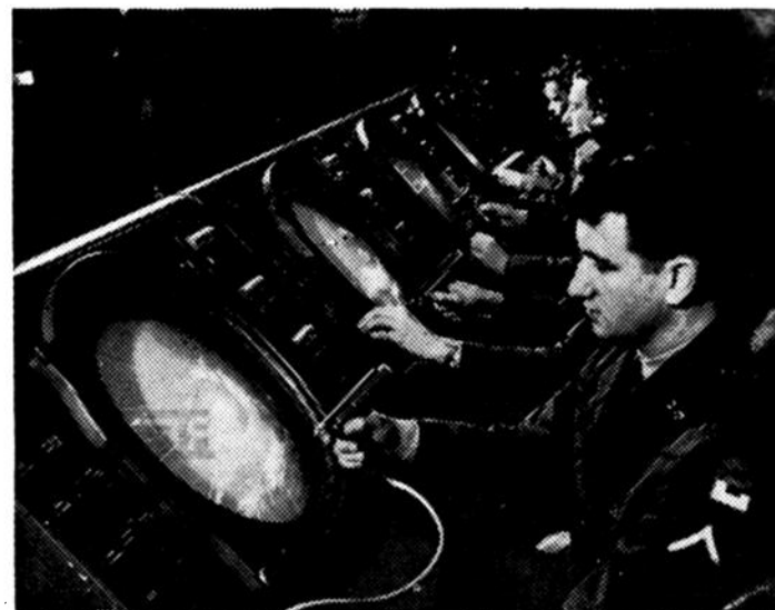
MISSILE MASTER SYSTEM — Electronic consoles, similar to these radar entry consoles in the system at Fort George G. Meade, Md., are the heart of the Missile Master system. Here, operators use photo-electric light guns placed against the screens to enter targets into the electronic tracking system.
