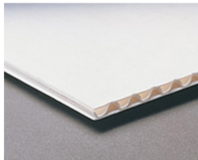
Figure 1-3: A typical Sandwich Structure. (Source: http://www.talasonline.com )
