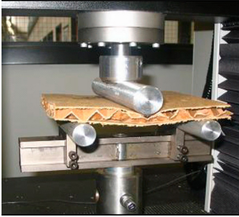
Figure 2-13: Sandwich Board Strength Test Setup. (Source: Industrial and System Engineering Dept. at Rutgers Univ.)
