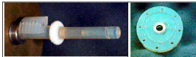
Figure 8-1: Previous sealing methods - Teflon Seal on FP shaft (L), Seal inside actuator cover (R).
