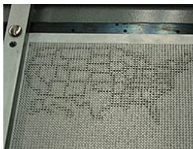
Figure 2-18: NIST Tactile Visual Display showing a map of the United States.
