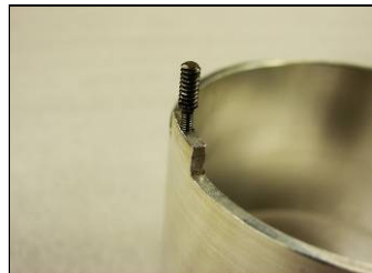
Figure 8-15: Threaded Attachment Point Assembled to Fixed Electrode
