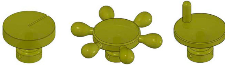
Three basic knob types – Disc, Lobed, Hand Wheel Surface Texture will be added to each for a total of six knob types.
