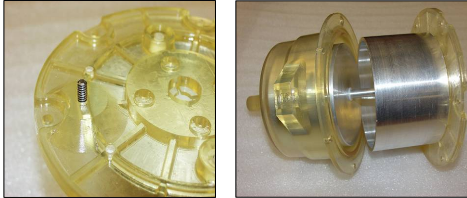
Figure 8-16: Cover assembled to Electrode (L) Electrode Inserted into Case (R)
