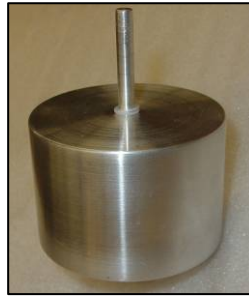
Figure 8-5: Rotating electrode, with attached output shaft
