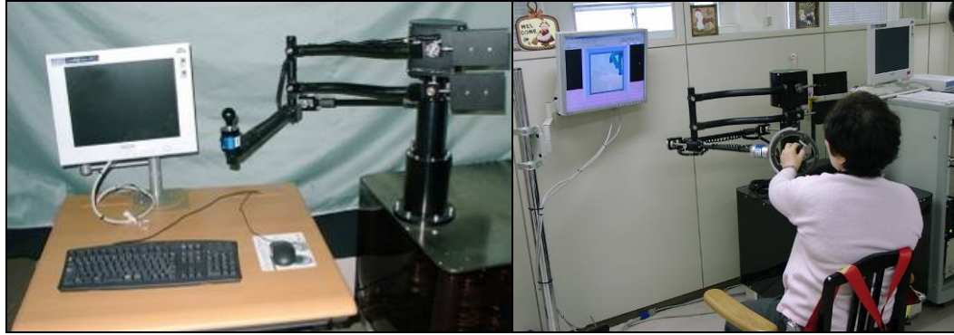
Figure 3-5: Force Display Device using electrorheological fluids.
