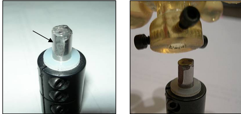
Figure 12-2: Extended Shaft with Flattened Edges (L) Attachment to Knob Base (R)
