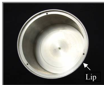
Figure 8-6: Bottom of electrode with attachment lip
