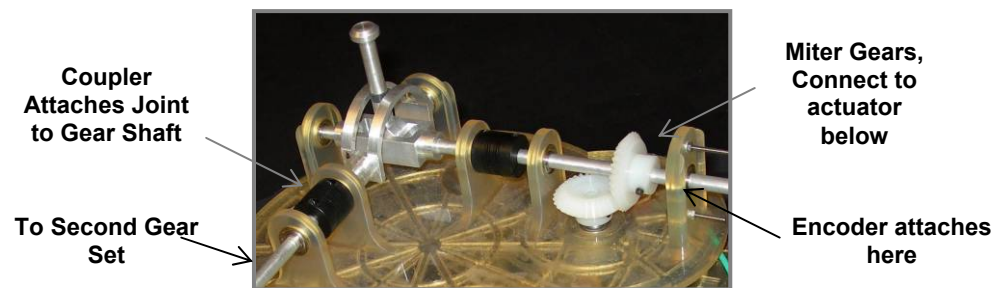
Figure 10-3: Miter Gear Assembly, Attaches Joint to Actuators
