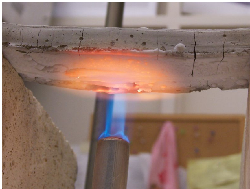
Figure 9: Swelling of the geopolymer glue
