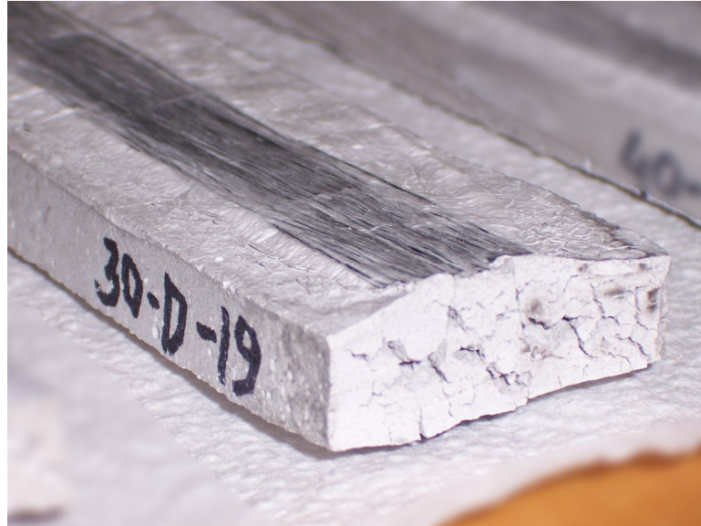
Figure 14: End cracking 1TC (30D19)
