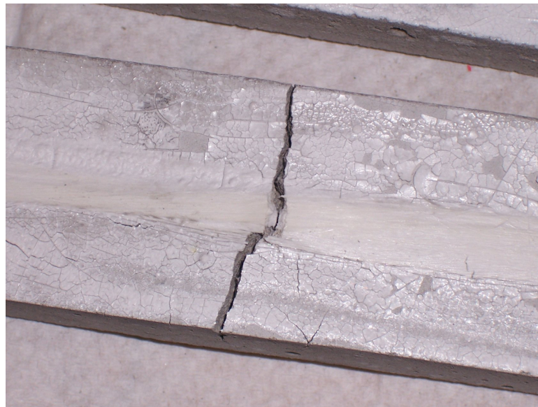
Figure 17: Structural failure caused by expanding geopolymer droplet
