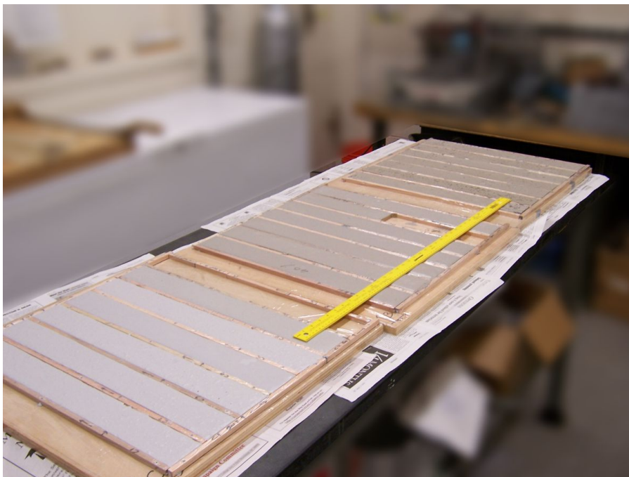
Figure 3: Wooden molds covered with Teflon® film
