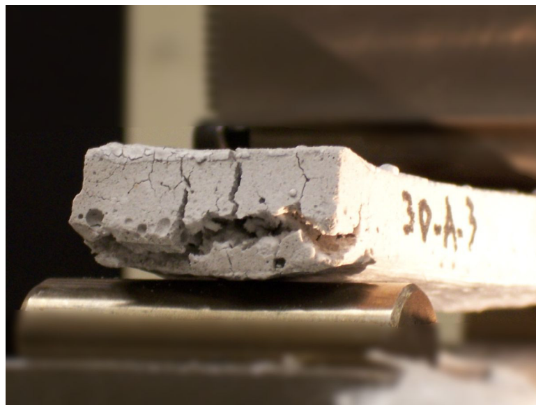
Figure 15: End cracking 2TC (30A3)
