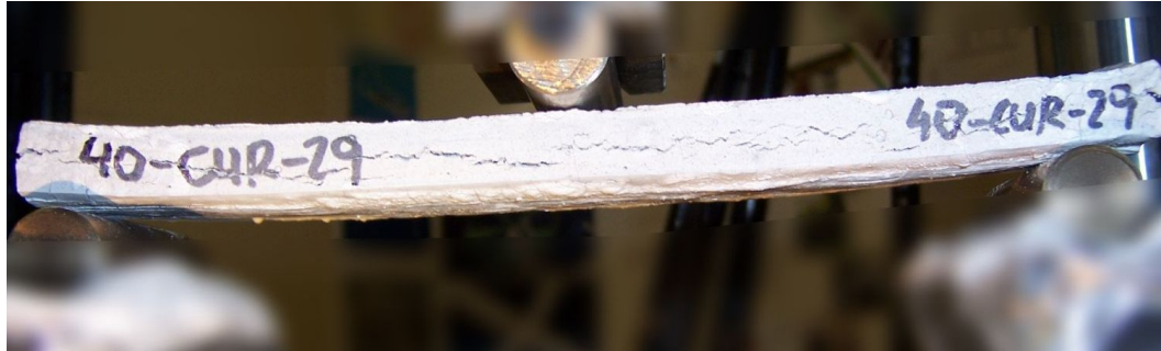
Figure 16: Longitudinal cracks 1TC (40cured29)
