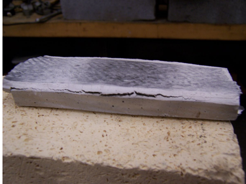
Figure 12: Longitudinal cracks formed underneath the reinforcing layer (40D20)
