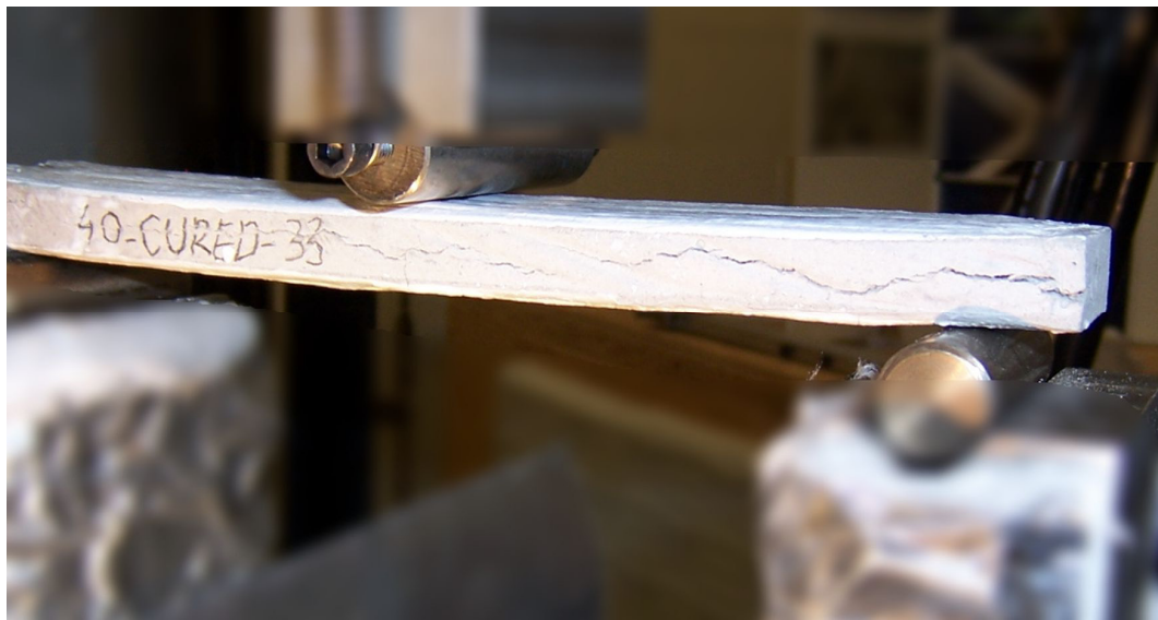
Figure 26: Longitudinal cracks appeared after the oven cycle (40cured33)
