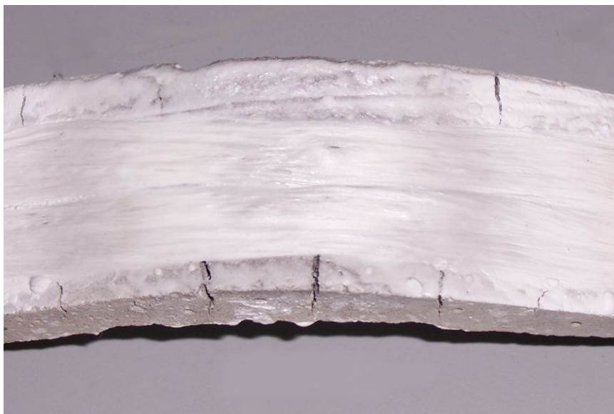
Figure 13: Cracks and melting of material surface area (50E28)
