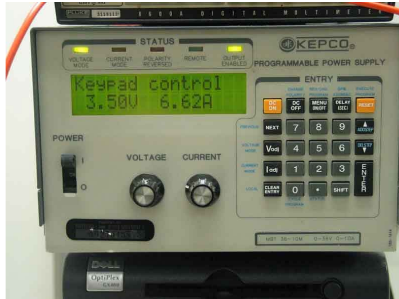
Figure 7.4 The programmable power supply
