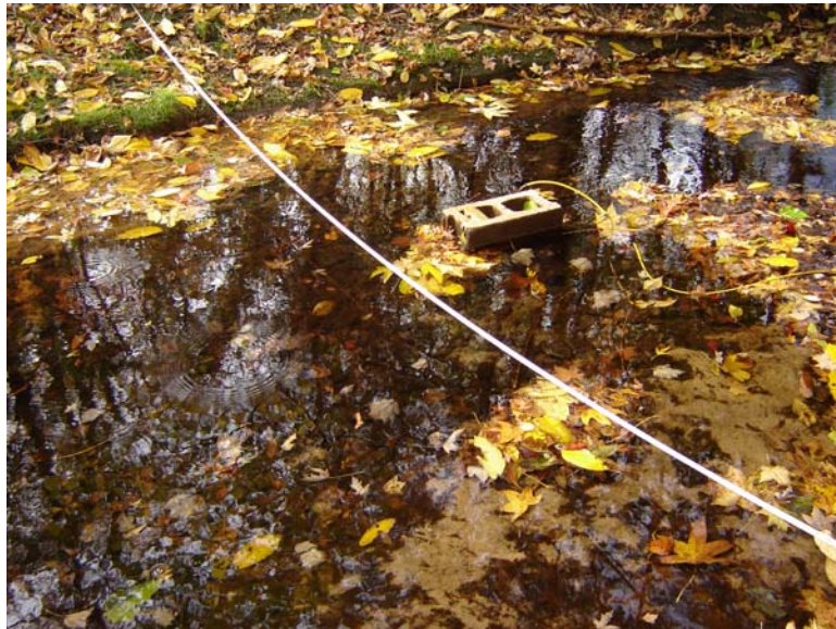
Figure 14: Pressure Transducer Deployed in the West Branch of the Pomepston Creek at Site 1
