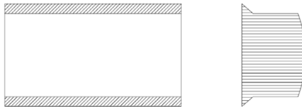
Figure 3.3 Shear stress distribution in a sandwich beam cross section
