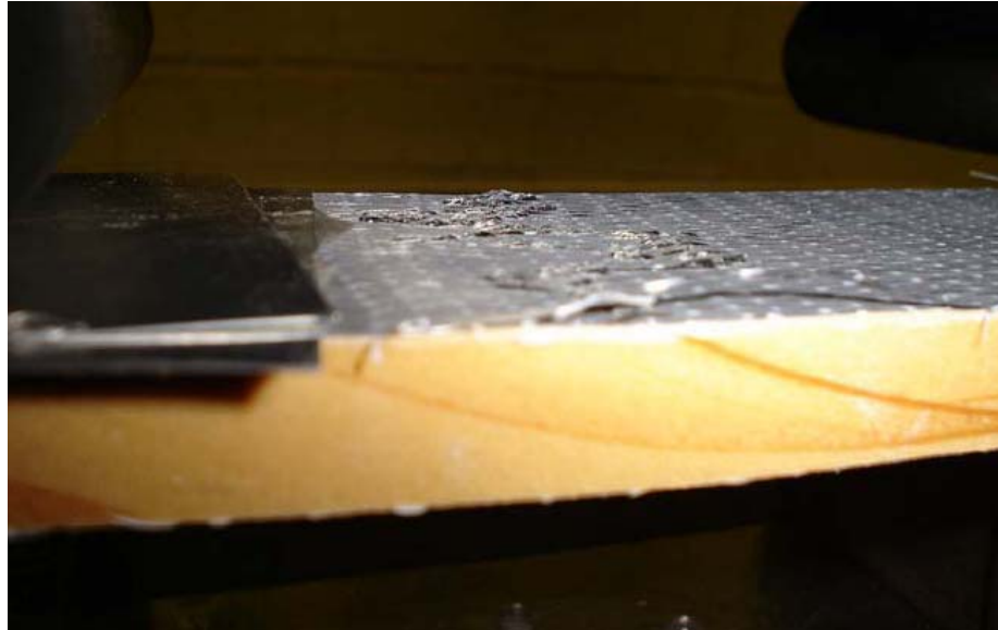
Figure 3. 28 Wrinkling failure for inorganic composite
