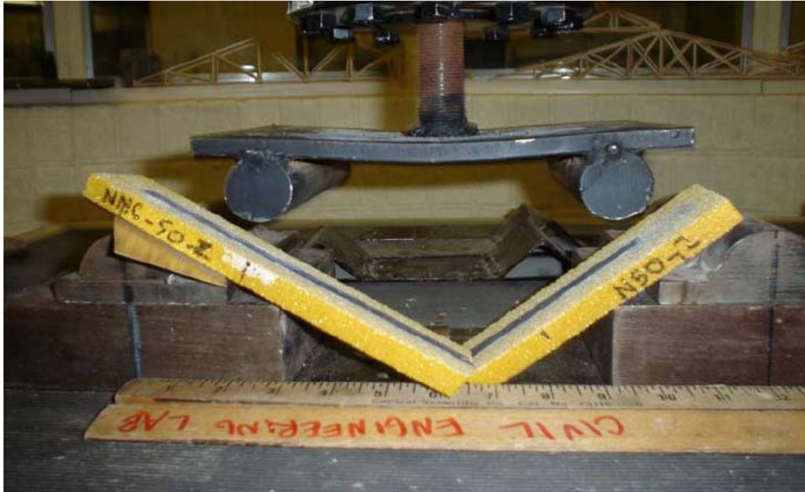
Figure 3.25 Tension split at midspan
