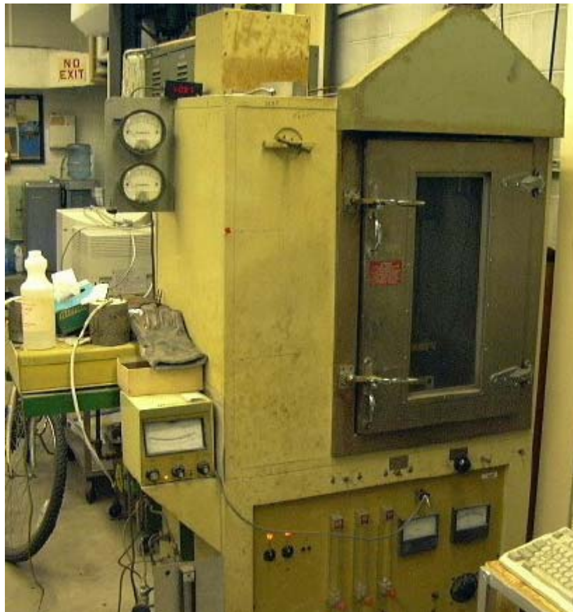
Figure 6.20 NBS testing setup (Papakonstantinou, 2003)
