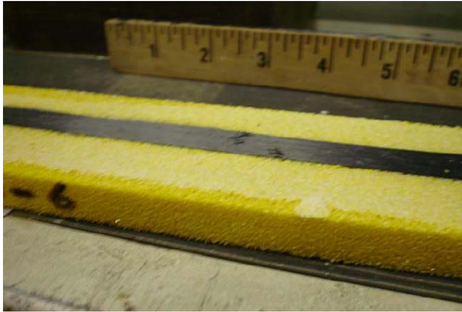
Figure 4.1 Wrinkling failure for inorganic composites
