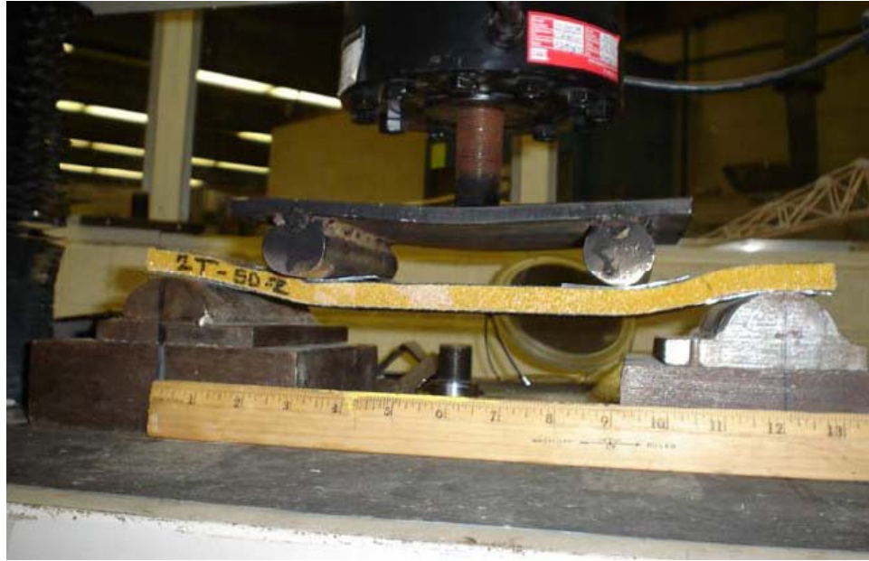
Figure 3. 26 Shear failure (near right support) and bearing failure (under left load roller)
