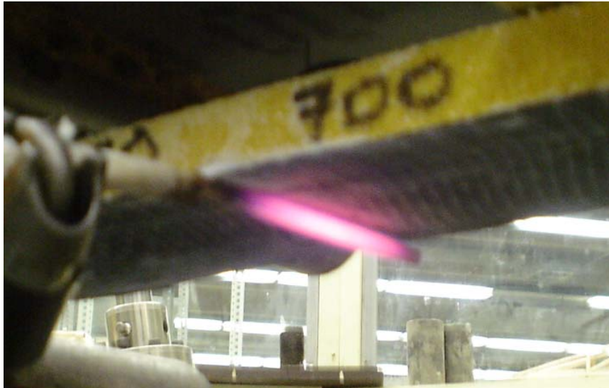
Figure 7.5 Heating element at 700°C
