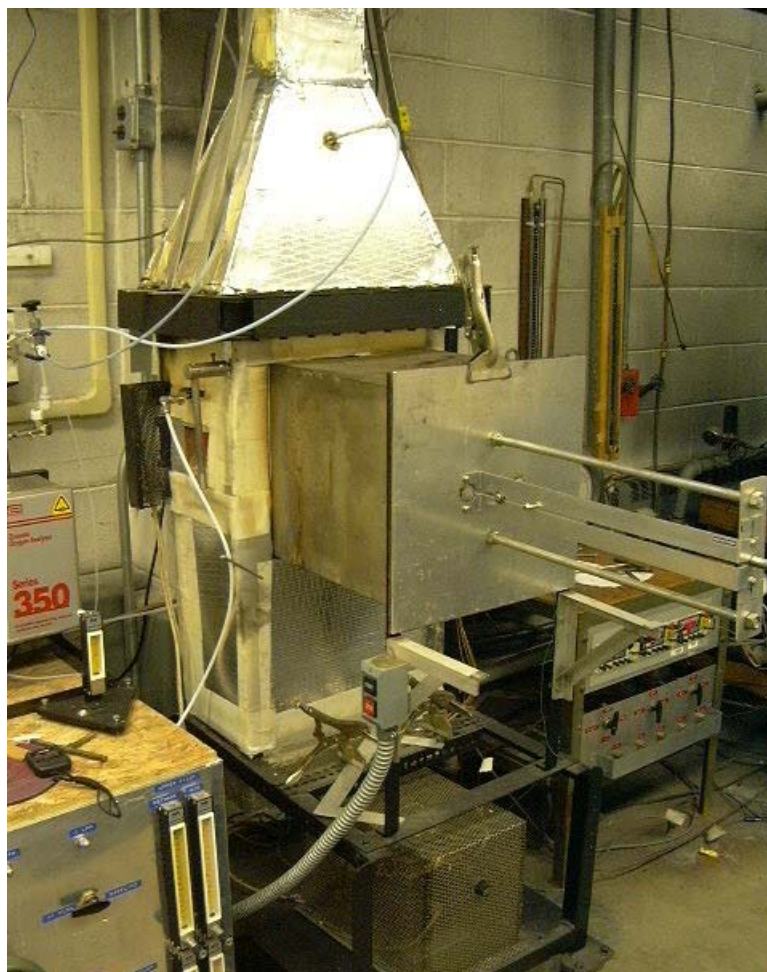
Figure 6.3 OSU heat release testing setup (Papakonstantinou, 2003)
