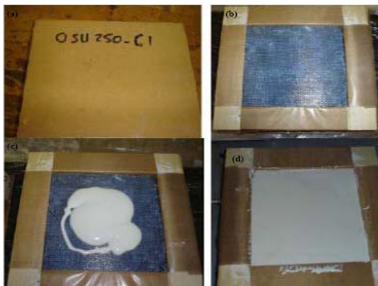
Figure 6.5 Samples preparation steps, (a) PVC foam core, (b) Core with unidirectional carbon in the mold, (c) Applying the coating (d) After coating application
