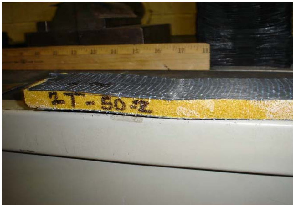
Figure 3. 27 Close-up for bearing failure under left load roller
