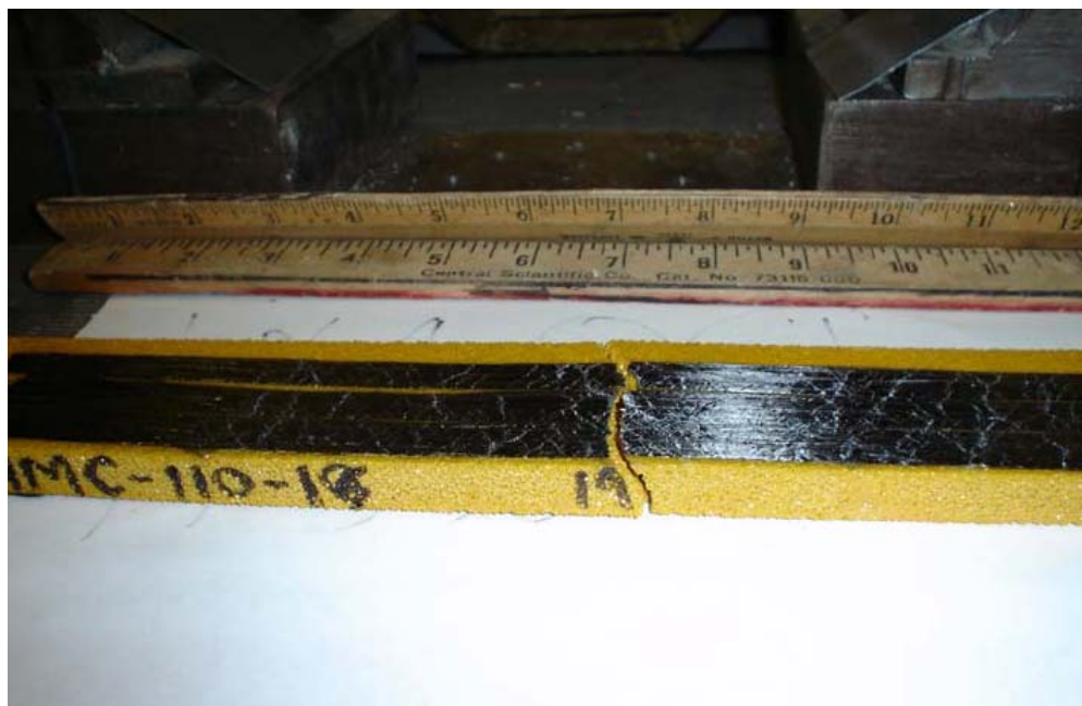
Figure 3. 29 Wrinkling and tension splitting failure for organic composites
