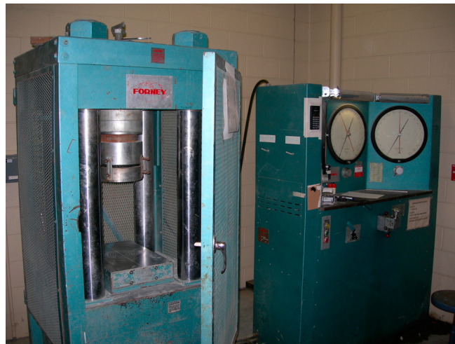
Figure 3.9. Forney 1-Million Pound Compression Machine
