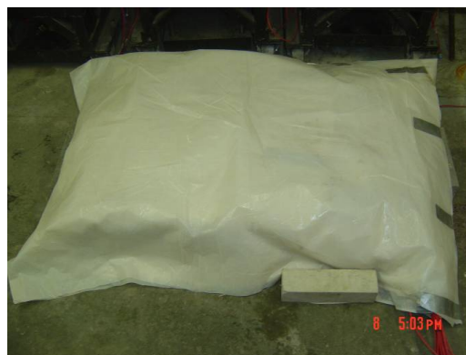
Figure 3.7. All Specimens Under Burlap and Polyethylene Sheet
