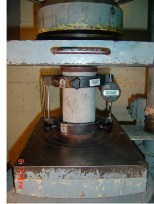
Figure 3.12. Modulus of Elasticity Test Setup
