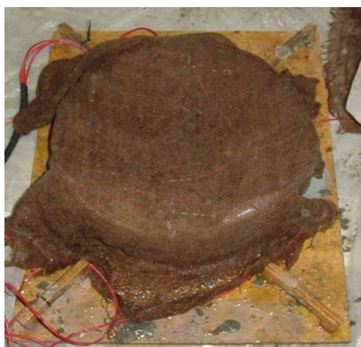
Figure 3.6. Restrained shrinkage specimen covered with wet burlap
