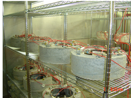
Figure 3.20. Close Up View of Rings in the Environmental Chamber
