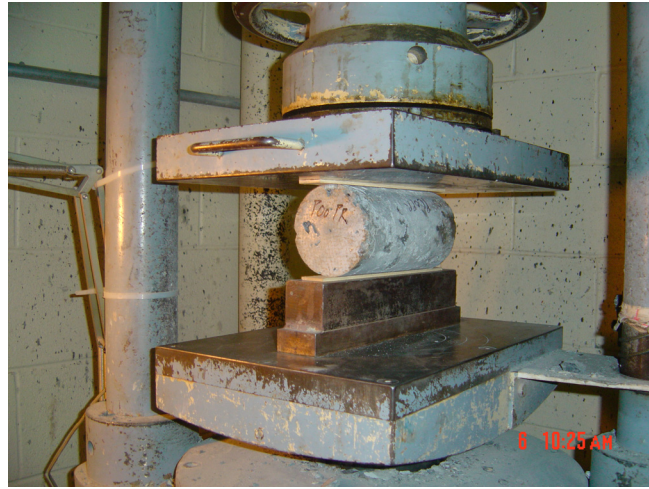
Figure 3.10. Splitting Tensile Strength Test Setup
