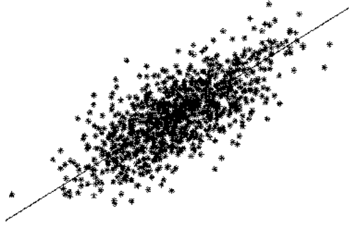
Figure 3.2: From [Hyvarinen, 1999]. The first principal component of a 2D dataset.
