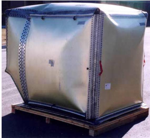
Figure 6.2: LD-3 luggage container deformed due to internal explosive loading [99].
