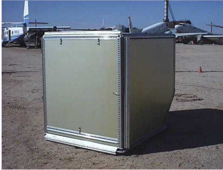
Figure 5.2: LD-3 luggage container with large plate (LP) geometry in front [99].
