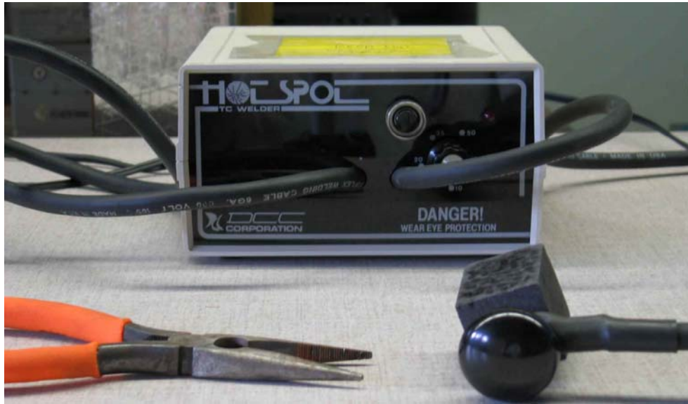
Figure 2.15: The Hot Spot Thermocouple Welder
