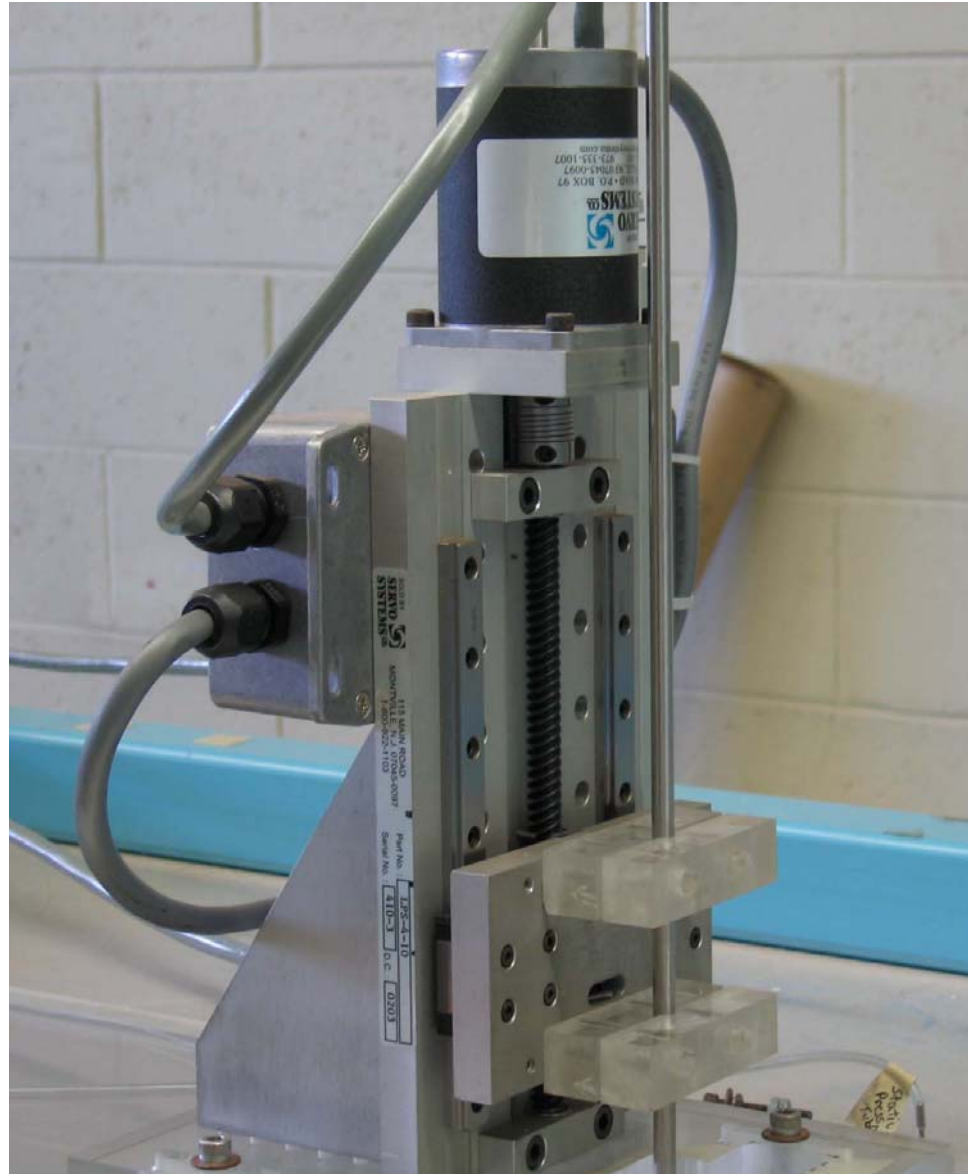
Figure 2.7: Transverse mechanism with motor
