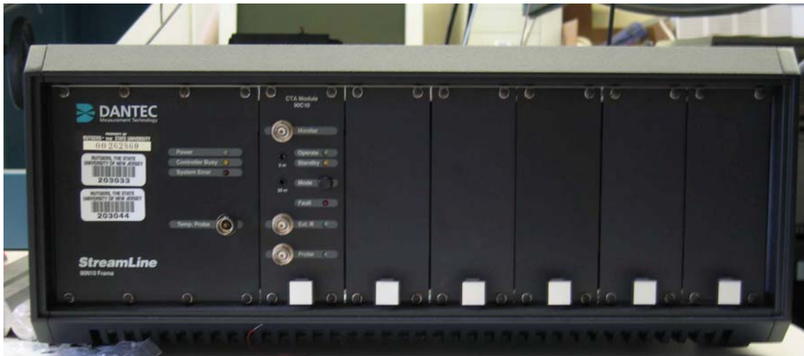
Figure 2.17: Streamline system Frame and CTA Module
