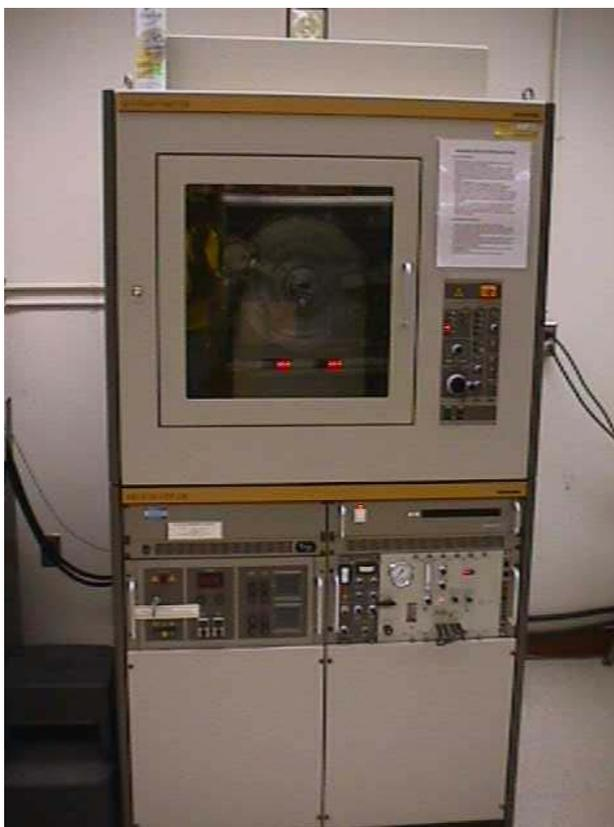
Figure 4.4.2: Siemens Goniometer (D500) X-Ray Diffractometer<sup>10</sup> (CCR 115)
