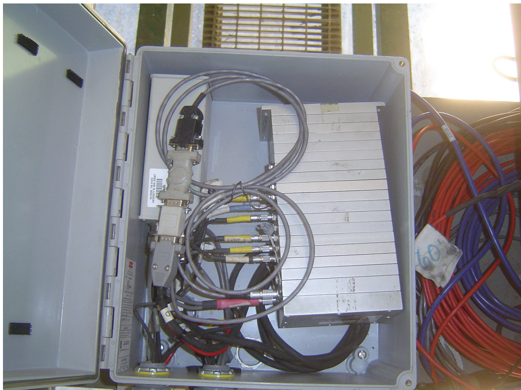
Figure 4.23 SoMat FCS2100 Data Acquisition System shown within protective enclosure
