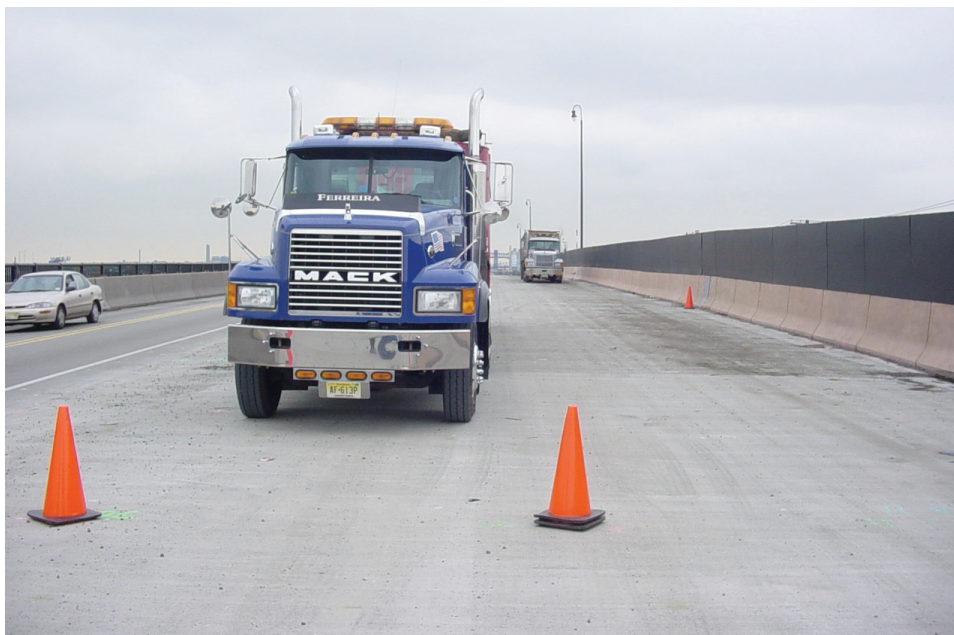
Figure 4.46 Stage II Controlled Load Testing 7/10/2003, single truck over G7 (Test 18)
