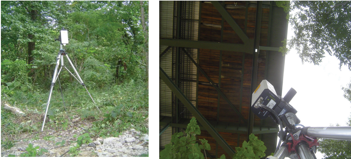
Figure 4.9 Laser Doppler Vibrometer for non-contact deflection measurement at a distance up to 300 feet.
