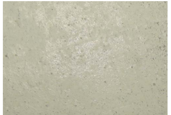
Fig. 3.33.2 shows no cracks with few depressions on the sample surface
