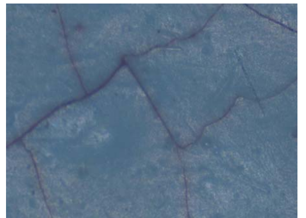
Fig. 3.3.3 digital microscopic picture showing block cracks (scale 25 μm)
