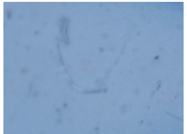
Fig. 3.42.3 digital microscopic picture showing no cracks with depressions (scale 25 µm)
