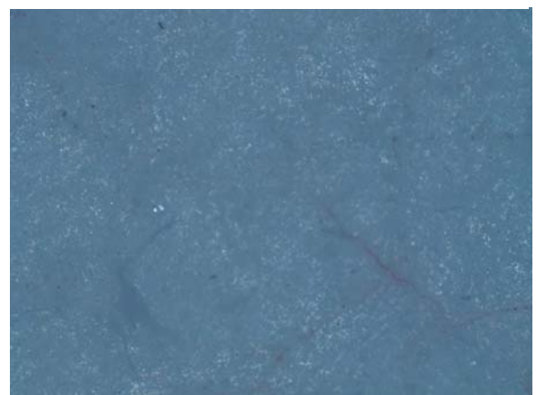
Fig. 3.26.3 digital microscopic picture showing fine cracks on the sample surface (scale 25 μm)
