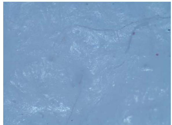
Fig. 3.6.3 digital microscopic picture showing minimal cracks (scale 25 \mu m)
