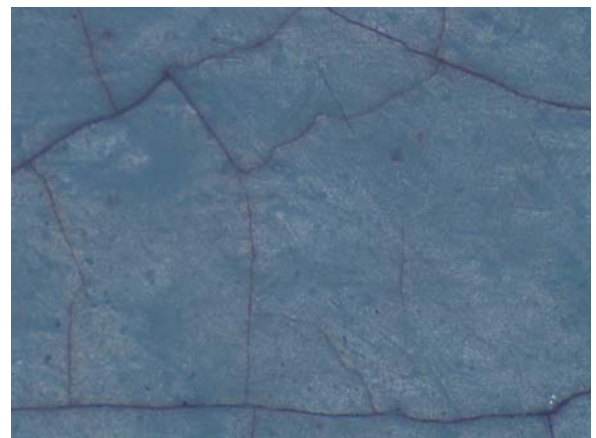
Fig. 3.19.3 digital microscopic picture showing large block cracks (scale 25 μm)
