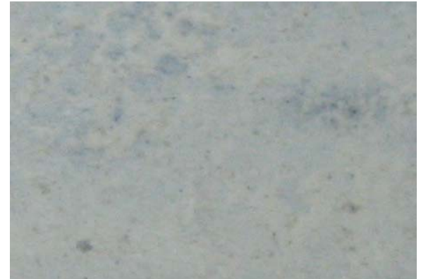
Fig. 3.22.2 shows almost no cracks with lots of depressions and holes
