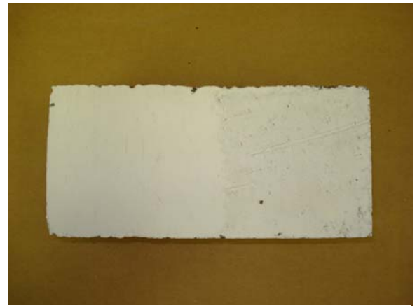
Fig. 3.7.1 shows mix no. 7 with two layers at the left side and one layer at the right side
