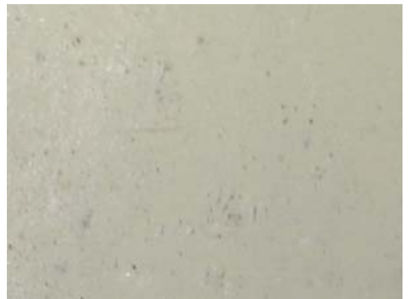
Fig. 3.30.2 shows small cracks and depressions all over the sample surface
