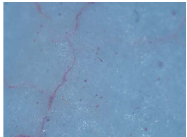
Fig. 3.28.3 digital microscopic picture showing longitudinal cracks (scale 25 μm)
