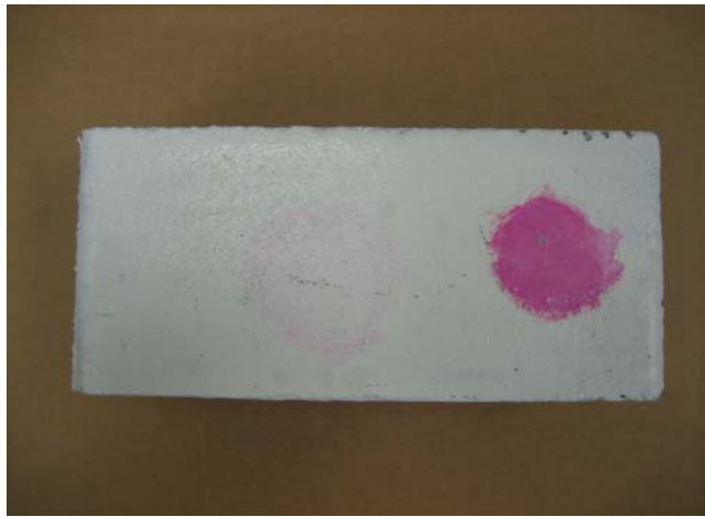
Fig. 5.1 show the difference in color tones of the dye when it was applied on a fresh mix and after the mix was cured
