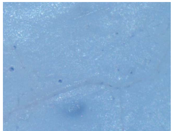
Fig. 3.20.3 digital microscopic picture showing minimal depressions (scale 25 µm)
