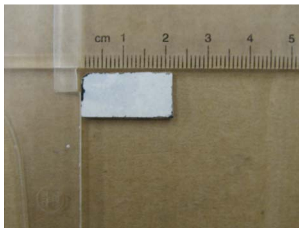
Fig 4.12 shows the XPS sample dimensions
