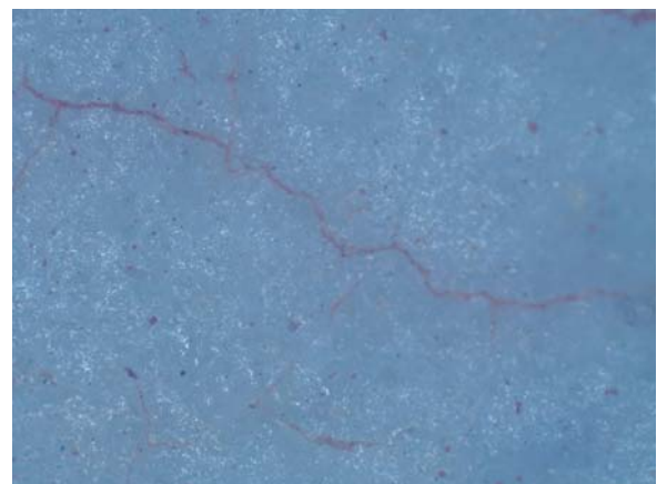
Fig. 3.25.3 digital microscopic picture showing diagonal cracks (scale 25 µm)
