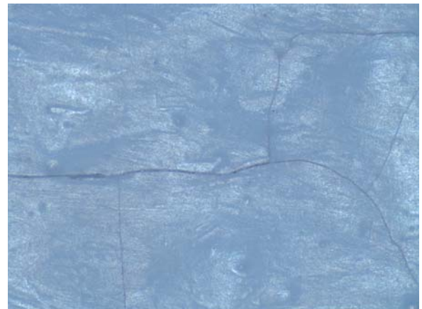
Fig. 3.14.3 digital microscopic picture showing block cracks (scale 25 \mu m)
