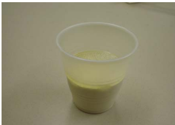
Fig 2.4 shows the coating mix sample placed in a plastic cup to measure the setting time
