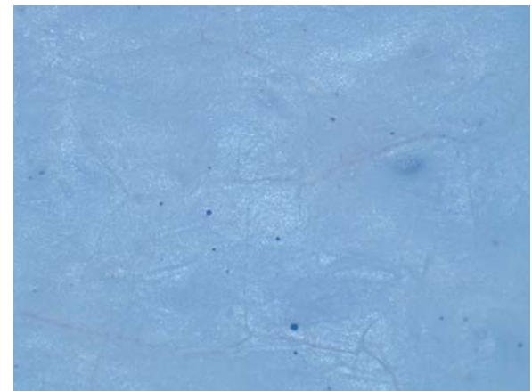
Fig. 3.22.3 digital microscopic picture showing very fine cracks < 1 \mu m (scale 25 \mu m)
