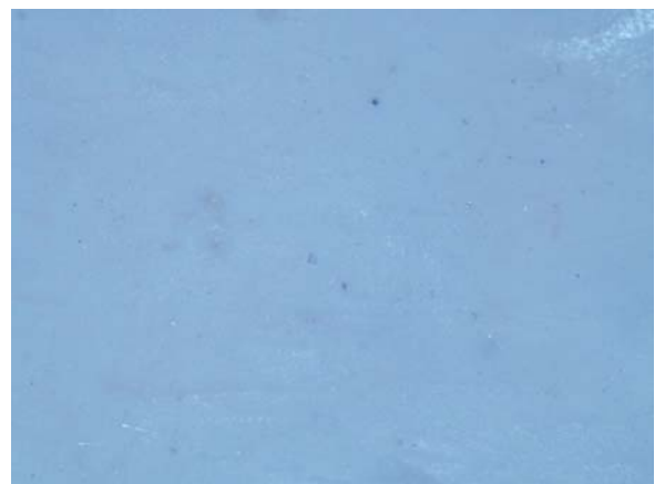
Fig. 3.17.3 digital microscopic picture showing no cracks (scale 25 μm)
