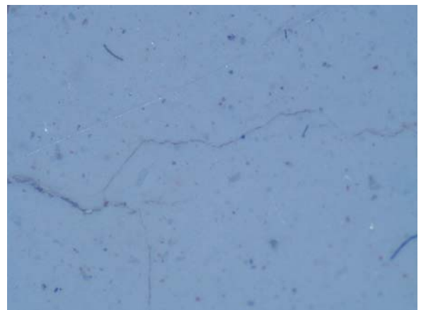
Fig. 3.48.3 digital microscopic picture showing small to medium size transverse cracks (scale 25 \mu m)
