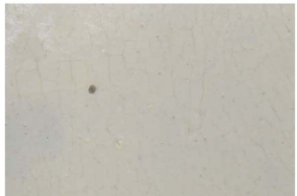
Fig. 3.31.2 shows cracks all over the sample surface
