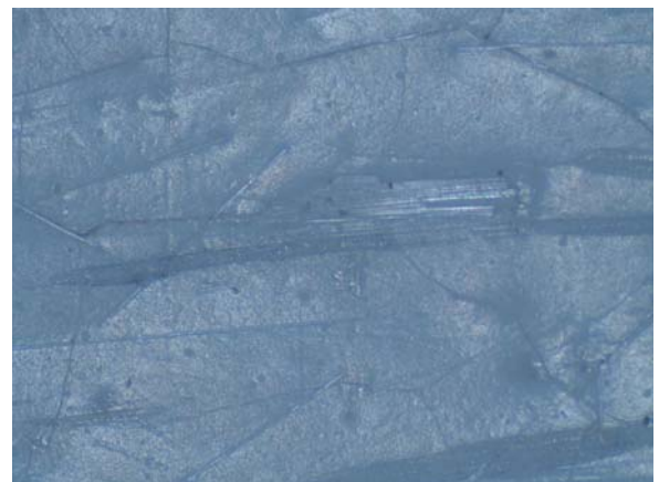
Fig. 3.38.3 digital microscopic picture showing cracks and heavy depressions (scale 25 μm)
