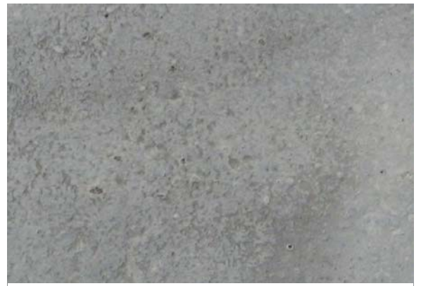
Fig. 3.21.2 shows almost pot holes and depressions all over the sample surface
