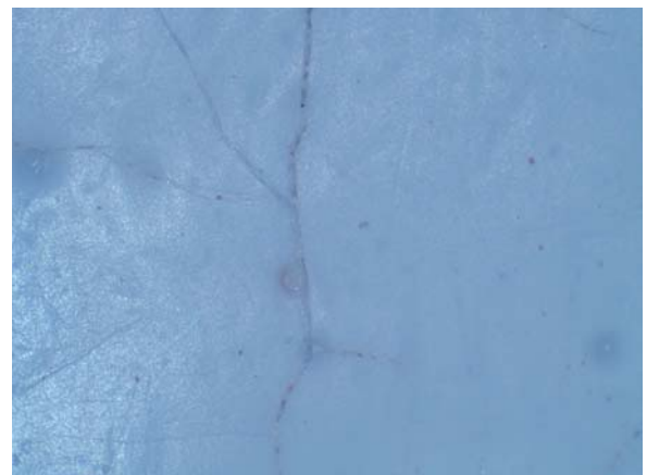
Fig. 3.31.3 digital microscopic picture showing transverse cracks (scale 25 μm)
