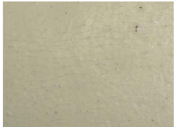
Fig. 3.14.2 shows the major cracks in the sample surface
