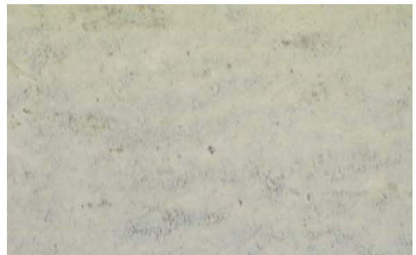
Fig. 3.6.2 shows no cracks under visual observation
