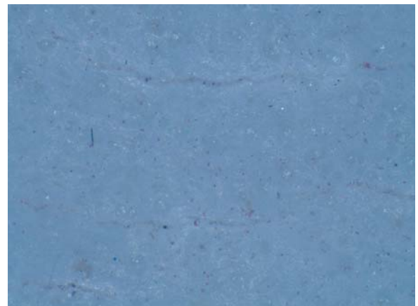
Fig. 3.13.3 digital microscopic picture showing very fine cracks < 1 \mu m (scale 25 \mu m)
