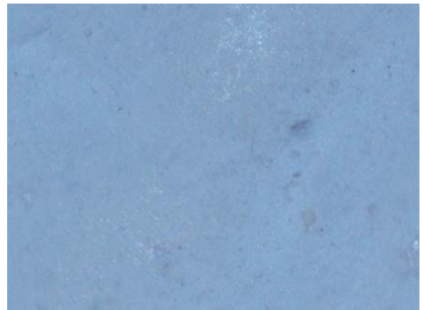
Fig. 3.34.3 microscopic picture showing no cracks with very few depressions (scale 25 µm)
