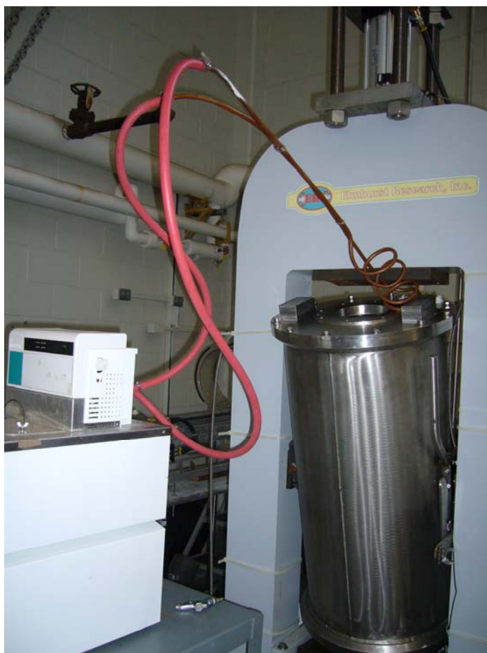
Figure 2.5 Experimental set up to heat the steel vessel using a circulating water bath.
