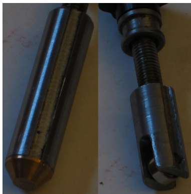
Figure 3.2: Steady Rest Inserts Original (Left) and Modified (Right).
