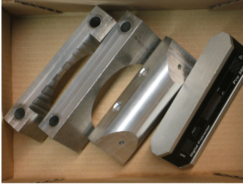
Figure 3.4: Vertical angle indicator and hold-down fixture
