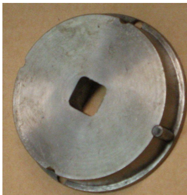
Figure A.5: Spanner Wrench for threaded lock ring
