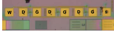
Figure 5.6 A test structure of MOSFET having three transistors in bunch with independent gate and drain.
