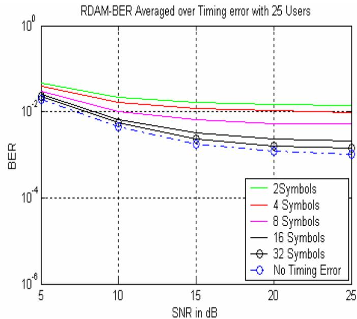
Figure 5.16: BER vs SNR for an ideal Rake Receiver,  $N_u=25$  users
