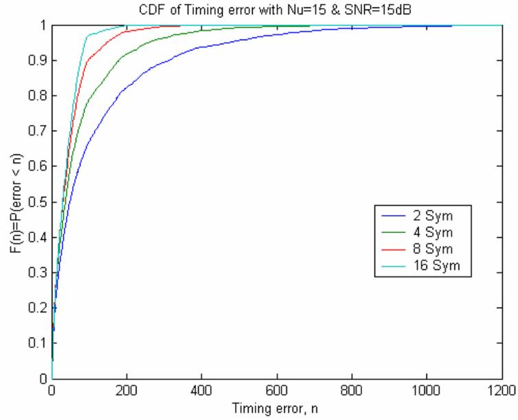
Figure 4.12: Timing Error CDF with  $\text{SNR}=15\text{dB}$ ,  $N_u=15$  Users
