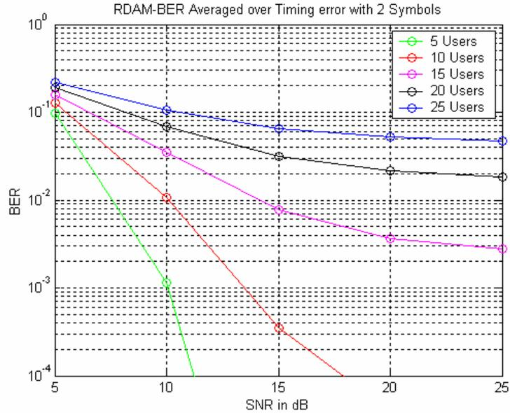
Figure 5.6: BER vs SNR for Increasing  $N_u$ , with  $M=2$  Symbols
