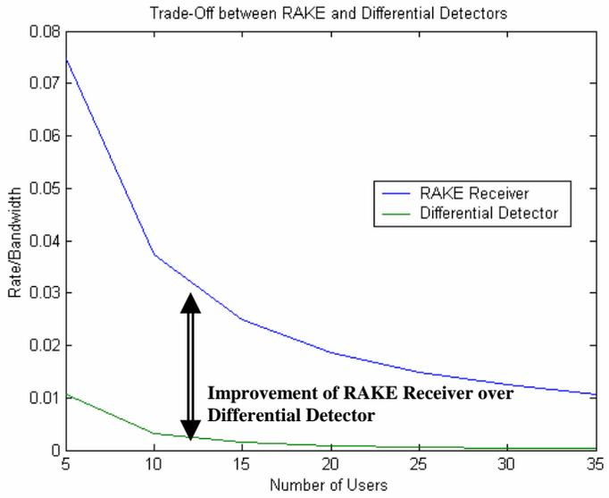
Figure 5.17: Rate-Bandwidth Ratio ( $R_b/W$ ) vs  $N_u$  comparison for fixed BER ( $10^{-2}$ ) (SNR~ with perfect timing acquisition)
