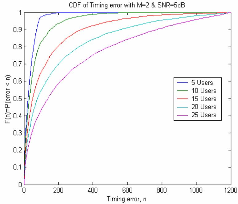
Figure 4.1: Timing Error CDF with M=2 Symbols, SNR=5dB
