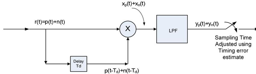
Figure 5.1: Standard DPSK/ Differential Detector Receiver Architecture
