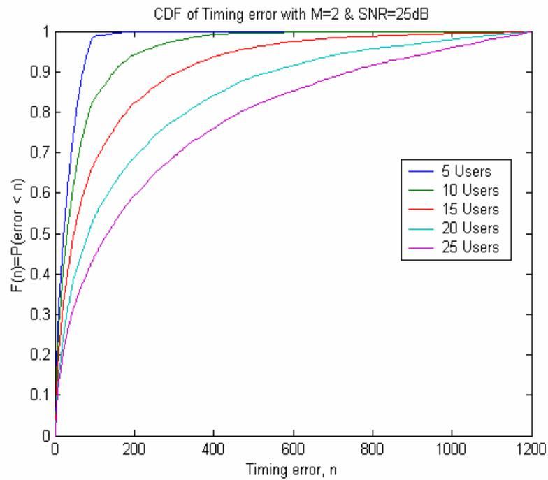
Figure 4.2: Timing Error CDF with M=2 Symbols, SNR=25dB
