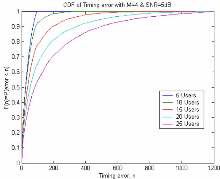
Figure 4.3: Timing Error CDF with M=4 Symbols, SNR=5dB
