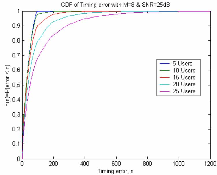
Figure 4.5: Timing Error CDF with  $M=8$  Symbols,  $\text{SNR}=25\text{dB}$
