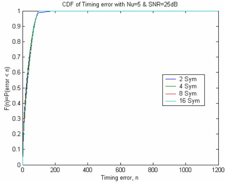
Figure 4.9: Timing Error CDF with SNR=25dB,  $N_u=5$  Users
