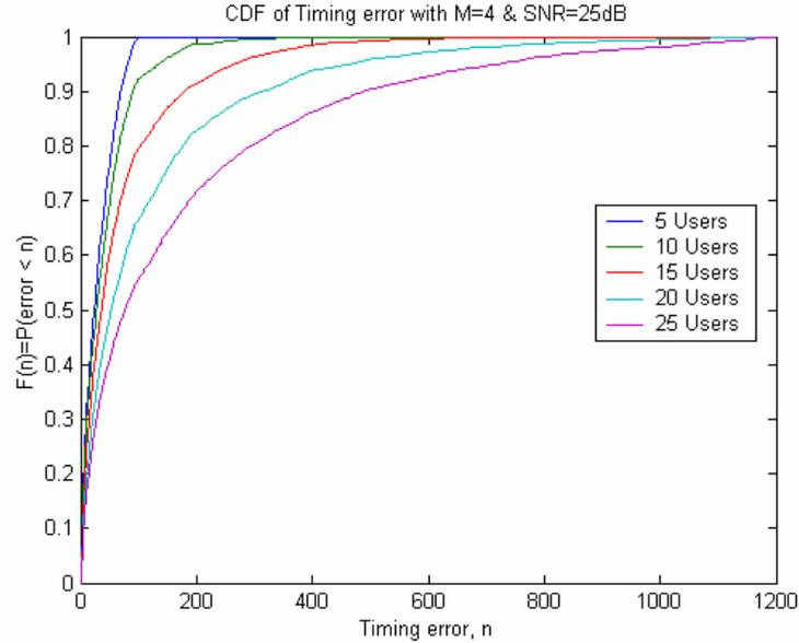
Figure 4.4: Timing Error CDF with M=4 Symbols, SNR=25dB
