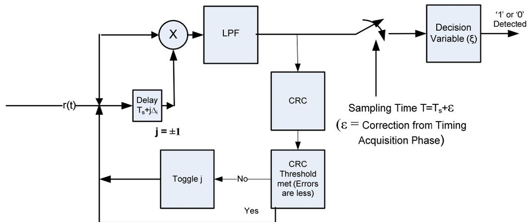
Figure 5.3: Modified DPSK Receiver Architecture#1
