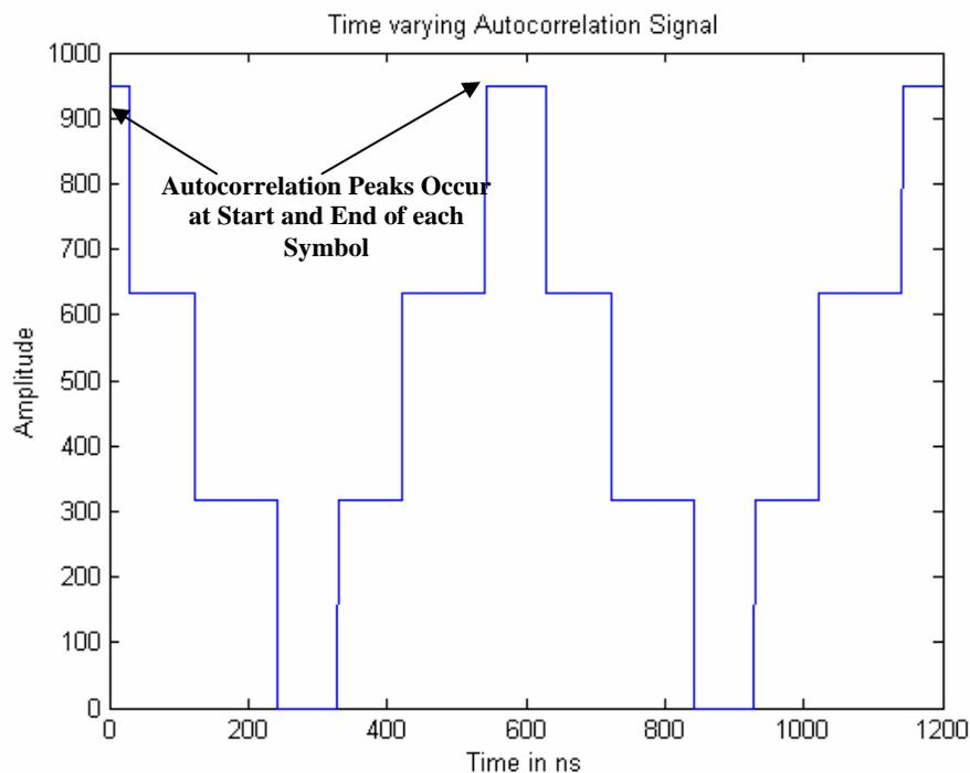
Figure 3.4: Time varying Autocorrelation with Half Symbol Delay
