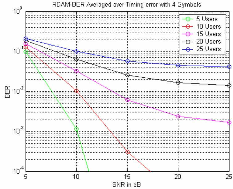
Figure 5.7: BER vs SNR for Increasing  $N_u$ , with  $M=4$  Symbols
