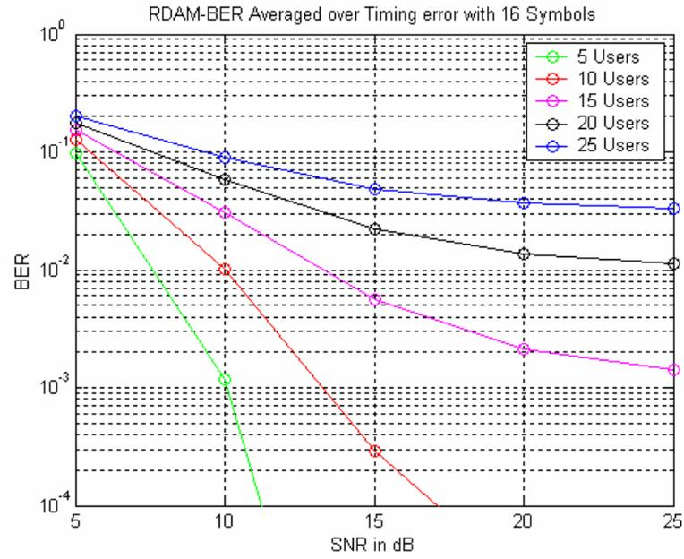
Figure 5.9: BER vs SNR for Increasing  $N_u$ , with  $M=16$  Symbols
