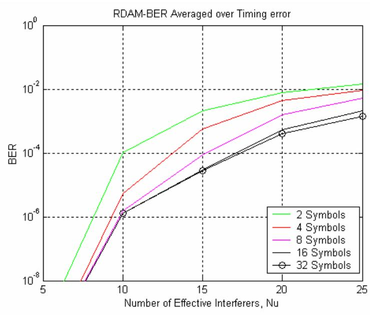
Figure 5.18: BER vs  $N_u$  for SNR=25dB, Rake receiver
