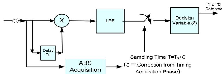
Figure 5.2: DPSK Receiver Architecture with Differential Signal Acquisition Phase
