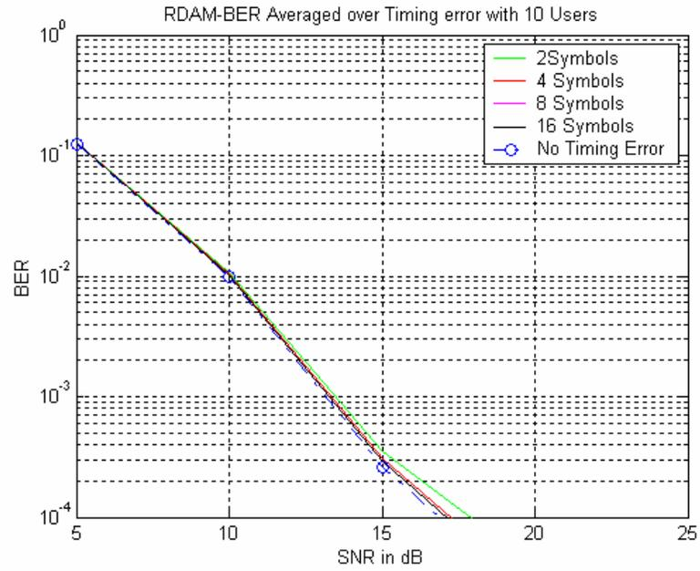
Figure 5.11: BER vs SNR for Increasing  $M$ , with  $N_u=10$  Users
