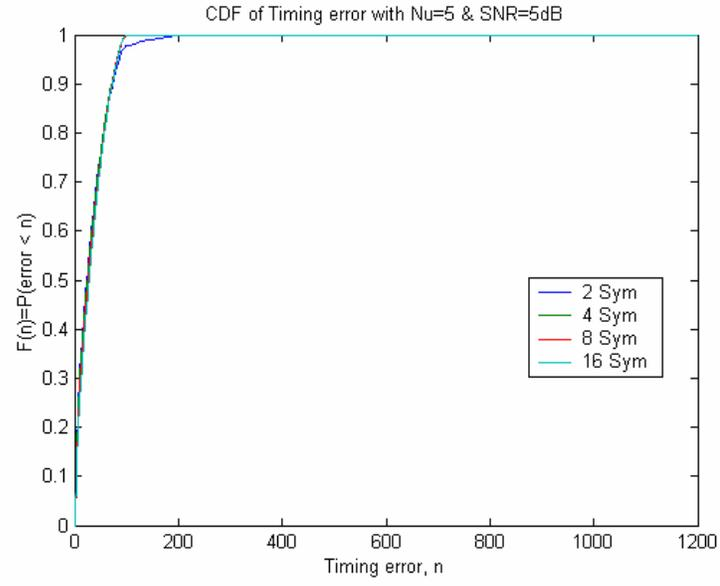
Figure 4.7: Timing Error CDF with  $\text{SNR}=5\text{dB}$ ,  $N_u=5$  Users
