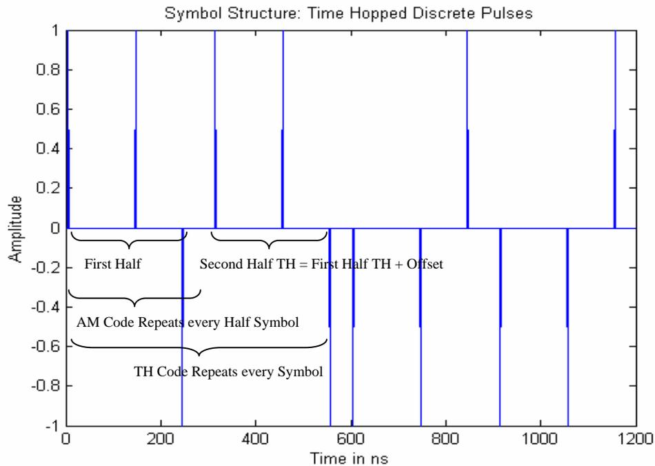
Figure 3.2: Symbol Structure of Time Hopped Discrete Pulse
