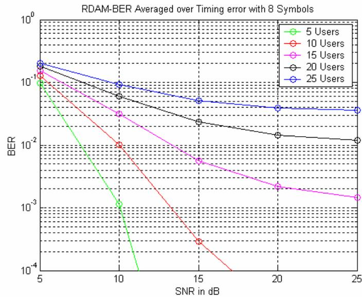
Figure 5.8: BER vs SNR for Increasing  $N_u$ , with  $M=8$  Symbols
