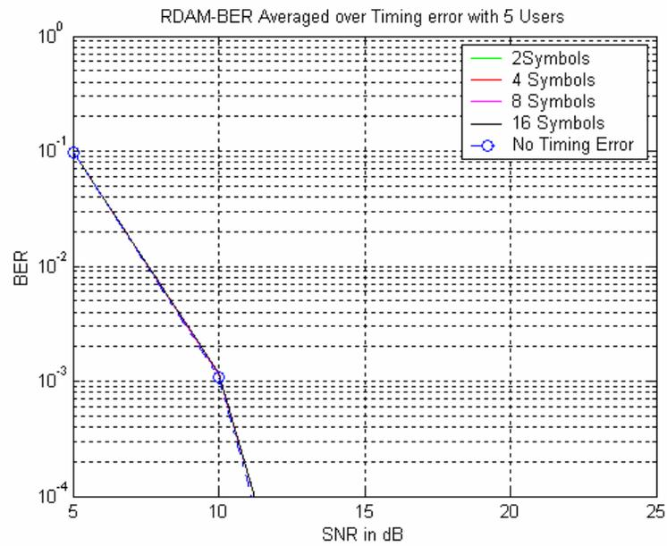
Figure 5.10: BER vs SNR for Increasing  $M$ , with  $N_u=5$  Users
