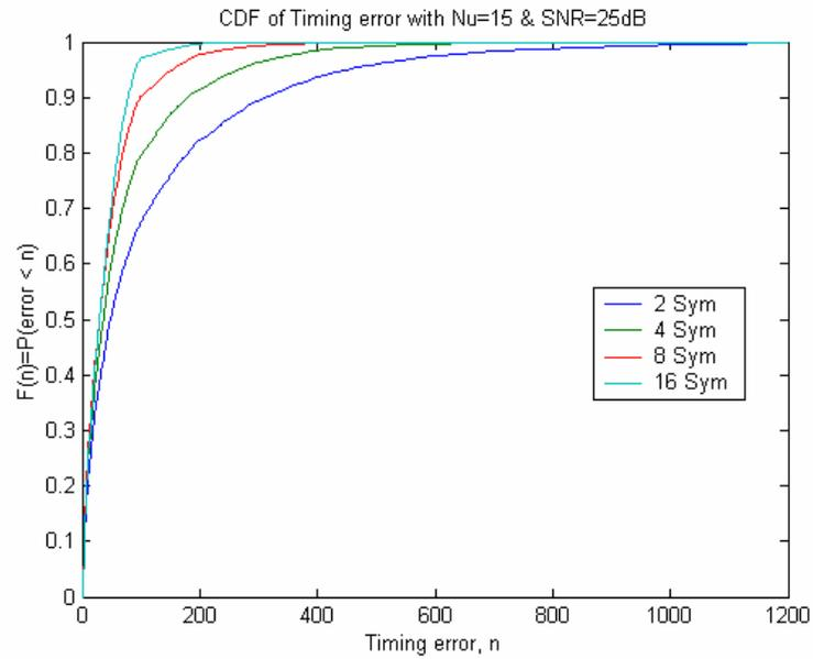
Figure 4.13: Timing Error CDF with  $\text{SNR}=25\text{dB}$ ,  $N_u=15$  Users
