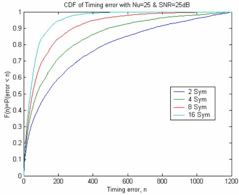
Figure 4.14: Timing Error CDF with SNR=25dB,  $N_u=25$  Users
