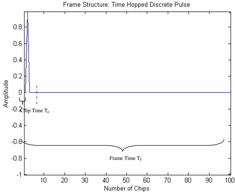
Figure 3.1: Frame Structure of Time Hopped Discrete Pulse
