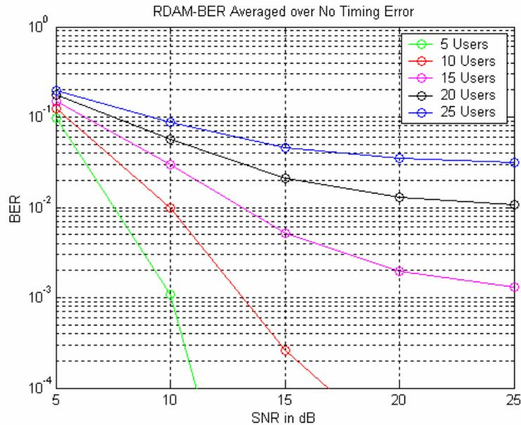
Figure 5.5: BER vs SNR for Increasing  $N_u$ , With No Timing Errors
