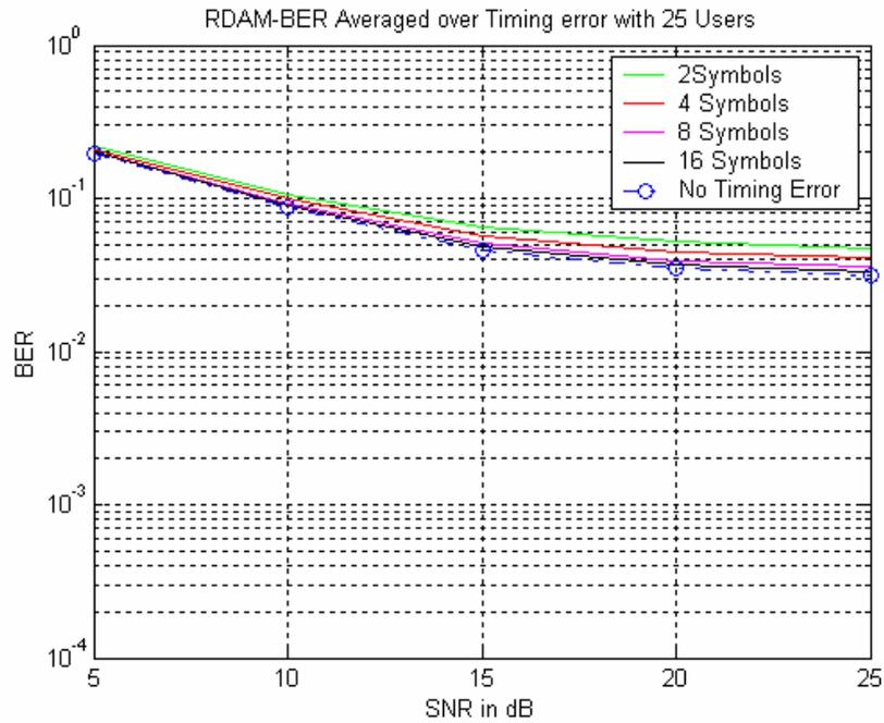
Figure 5.13: BER vs SNR for Increasing  $M$ , with  $N_u=25$  Users
