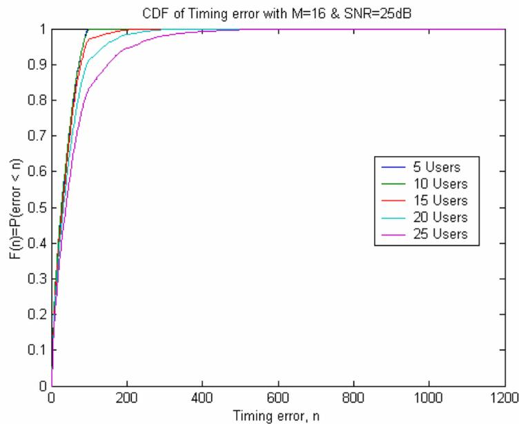
Figure 4.6: Timing Error CDF with  $M=16$  Symbols,  $\text{SNR}=25\text{dB}$
