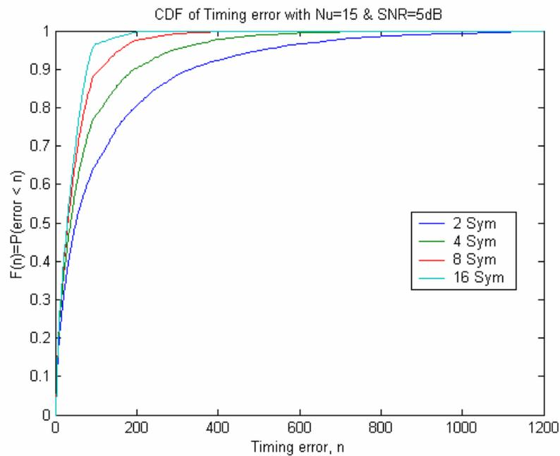
Figure 4.10: Timing Error CDF with SNR=5dB,  $N_u=15$  Users
