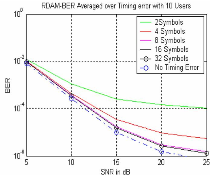
Figure 5.15: BER vs SNR for an ideal Rake Receiver,  $N_u=10$  users
