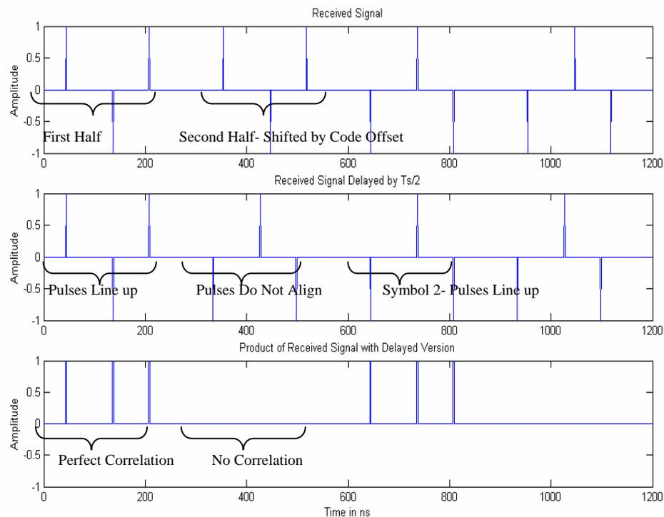
Figure 3.3: Delay and multiply process of received signal
