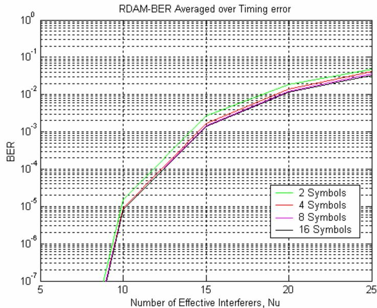
Figure 5.14: BER vs  $N_u$  for increasing  $M$
