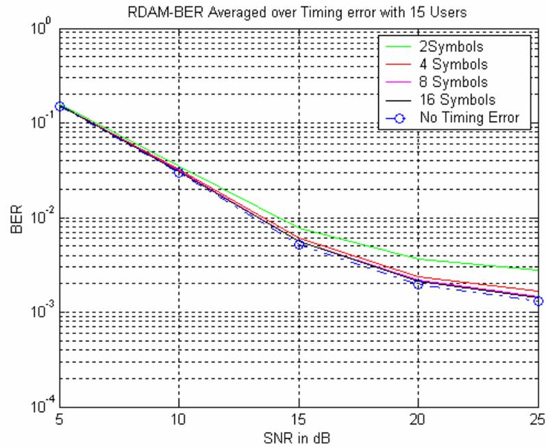
Figure 5.12: BER vs SNR for Increasing  $M$ , with  $N_u=15$  Users
