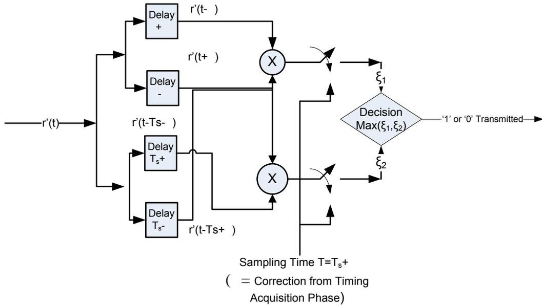
Figure 5.4: Modified DPSK Receiver Architecture#2
