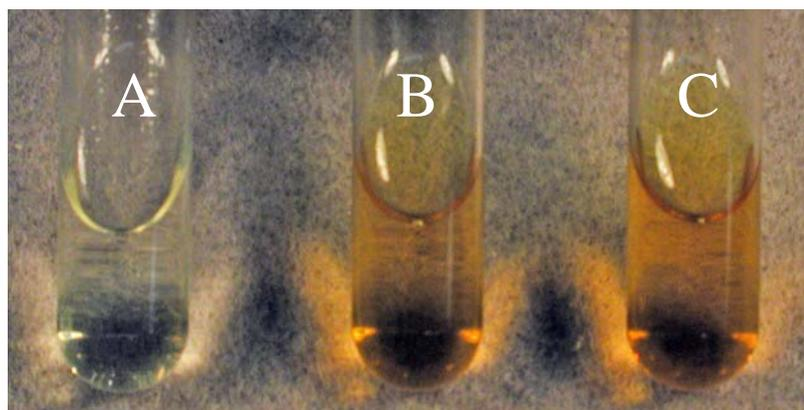
**Figure 7. Visible color change in titanium test solutions.** Relative to the control, (A) color change was immediately visible in the test solutions. Samples #5 (B) and #9 (C) from Table 1 are shown here. Yellow color indicates the presence of hydrogen peroxide at significantly higher levels. We hypothesize this result as a direct function of oxidative deaminase activity on naturally occurring levels of D-amino acids in the plant, or on alternative endogenous substrates.
