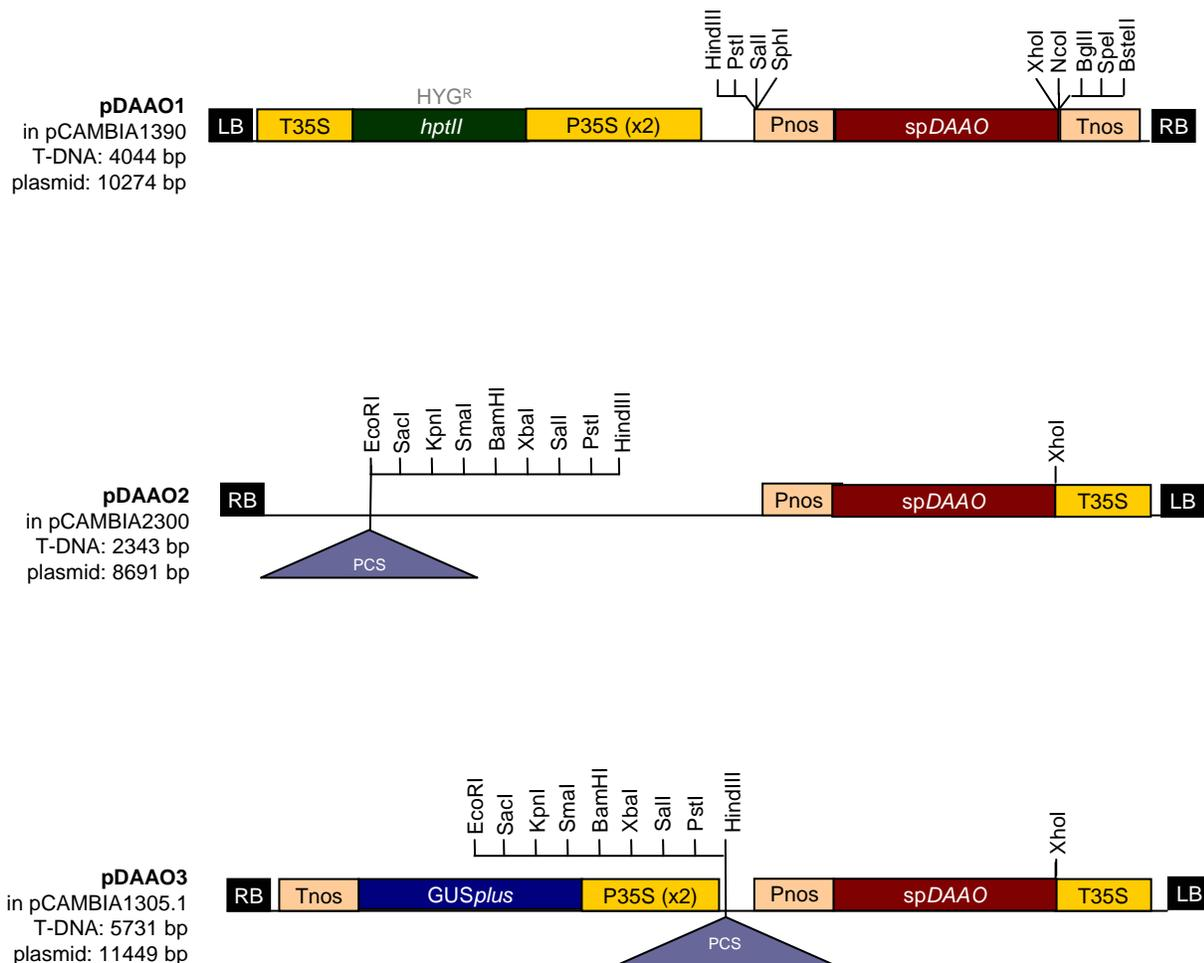
**Figure 4. Vectors.** The three binary vectors generated in this study contain the *spDAAO* driven by a nopaline synthase promoter. Additionally, pDAAO1 contains an *hptII* cassette conferring resistance to hygromycin. pDAAO3 contains a GUS construct to facilitate X-gluc staining. pDAAO2 and pDAAO3 contain the pUC18 polycloning site to facilitate insertion of future genes of interest.
