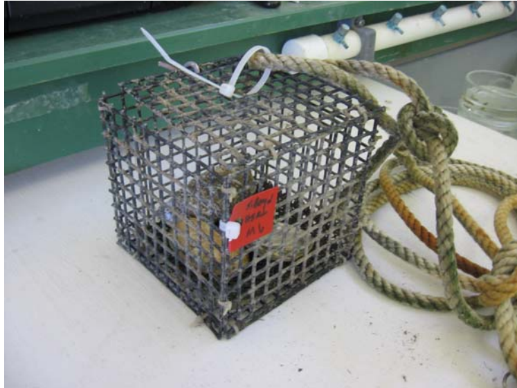
Figure 2.2 Wire-mesh cage deployed in the Maurice River, NJ to assess the affinity of S. laticauda for biologically fouled structures.
