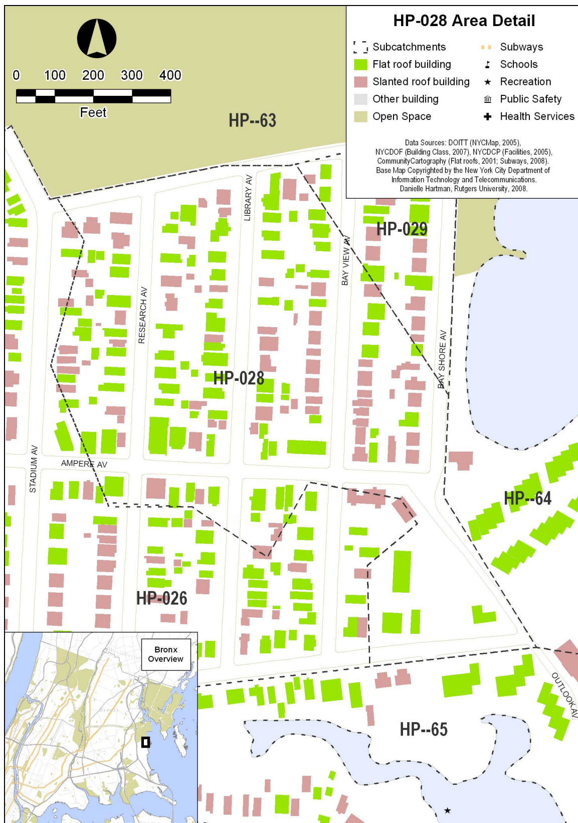
Figure 47. Map of HP-028 subcatchment. This outfall ranked third most sensitive overall to modeled green roof scenarios.
