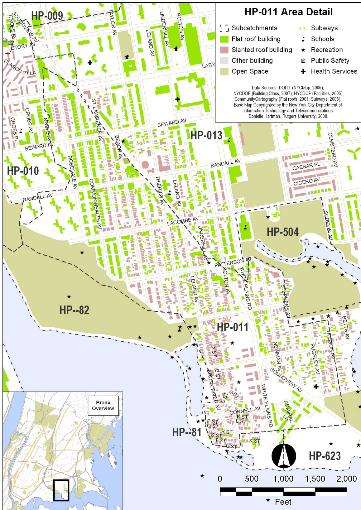
Figure 42. Map of HP-011 subcatchment. This Tier 1 outfall produced the fourth most Bronx CSOs by volume. It showed a strong response to modeled green roofs scenarios, highly sensitive to volume reduction.
