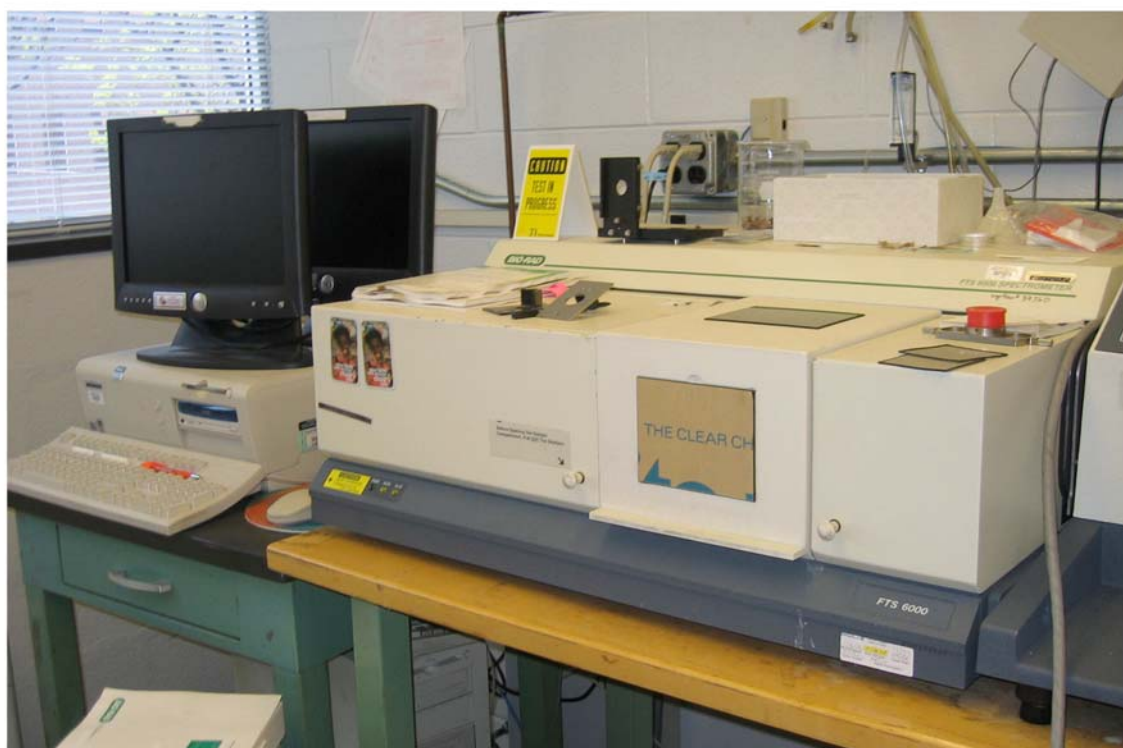
Image 4. Apparatus for examining infrared spectrum of vapor phase above 0.1 M potassium cyanide solution.
