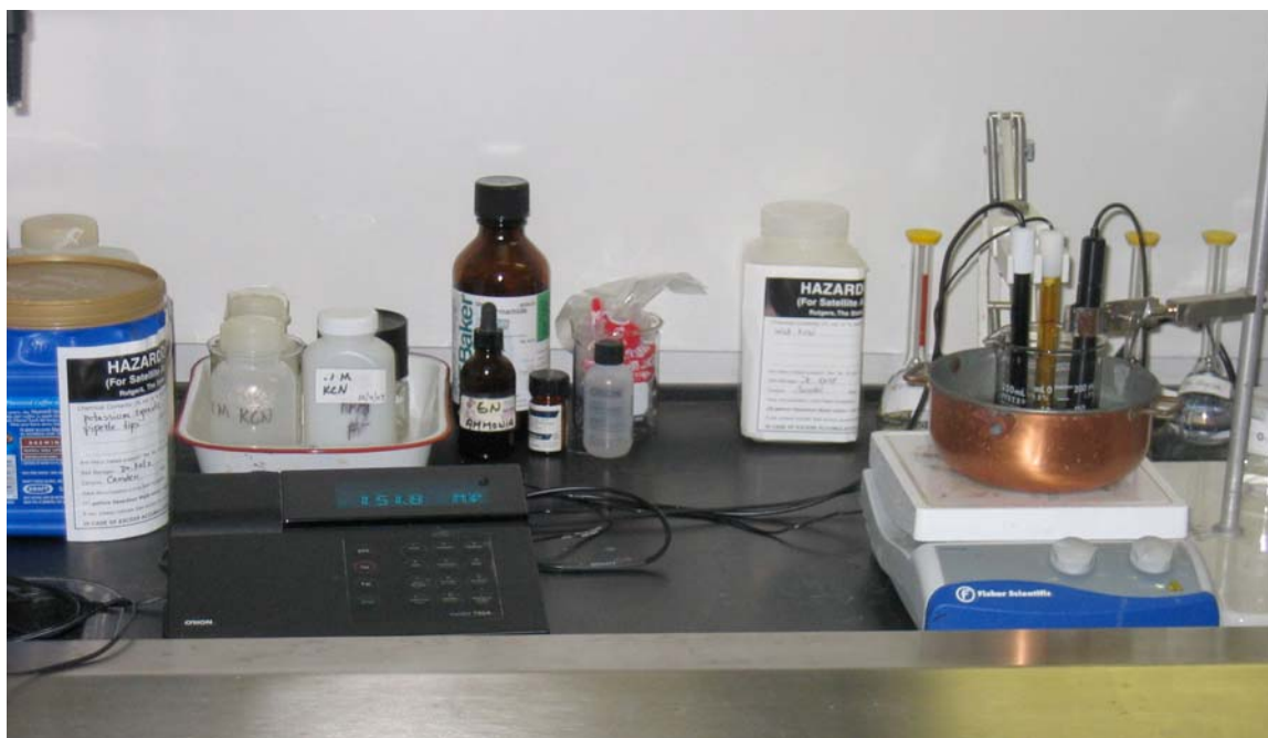
Image 2: Detail of experimental setup including electrodes, digital analyzer and standard solutions.
