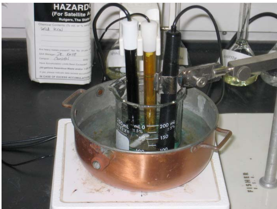
Image 3: Detail of electrodes immersed in reaction solution.
