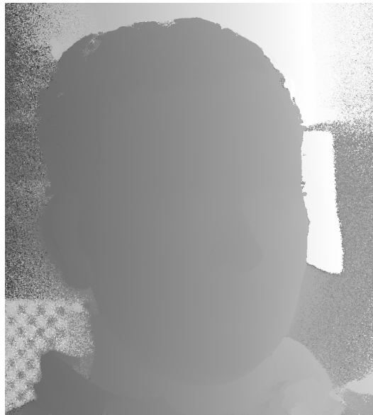
Figure 2.16: Stripe image of the front view of the face. Each pixel has been assigned an intensity equal to its stripe id divided by 256.
