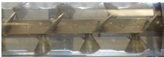
Figure 2.2.2: Convective Design of the Continuous Mixer
