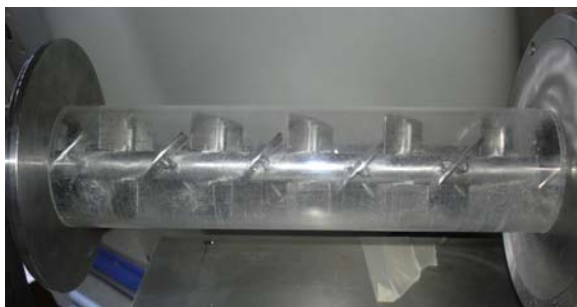
Figure 4.2 Detail of the impeller design in the continuous blender used for PEPT experiments
