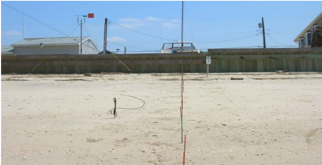
Figure 6 The control site with a bulkhead above normal spring high water and the anemometer and wind vane located on the bulkhead. A pressure transducer is visible on the foreshore.
