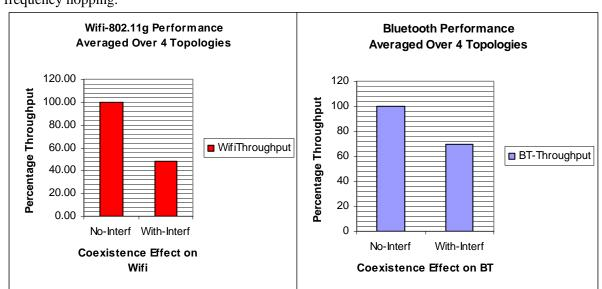
Fig 10(a) Coexistence Effect on WiFi session throughput (b) Effect on Bluetooth throughput
