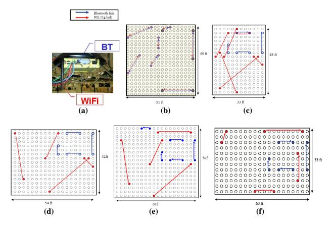
Fig. 9 Experiment Scenarios 9(a) Physical ORBIT multi-radio node 9(b - f) Evaluation Scenarios/topologies 1 through 5
