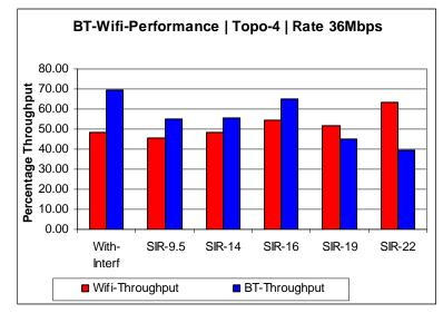
Fig. 16 Sensitivity of SIR\_link\_budget around 16dB for fixed rate 36Mbps
