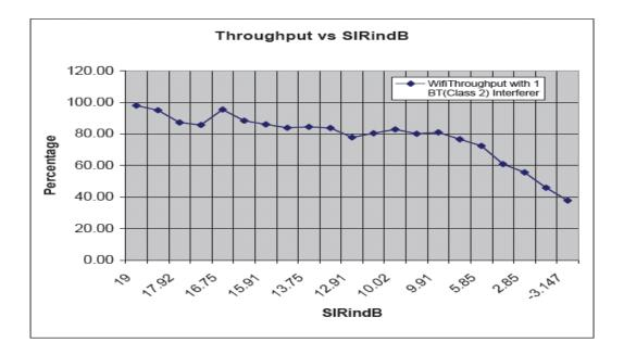
Fig. 7 Throughput vs Distance based SIR curve for 802.11g with BT (Class 2) Interferer.
