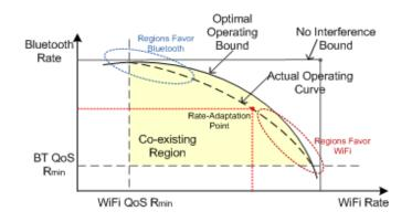
Fig. 5 Coexistence Region of Operation for BT-Wifi
