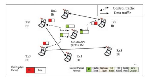
Fig. 6 SIR-BT Rate Adaptation for Wifi/BT Coexistence.
