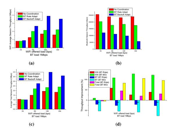
Figure 12 Experiment results for Throughput vs. WiFi loading rate. (a) WiFi session throughput (b) BT throughput (c) Average total network throughput (d) Throughput improvement for each case
