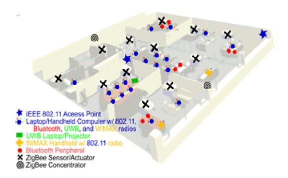
Fig. 1 SOHO scenario for multi-radio co-existence.
