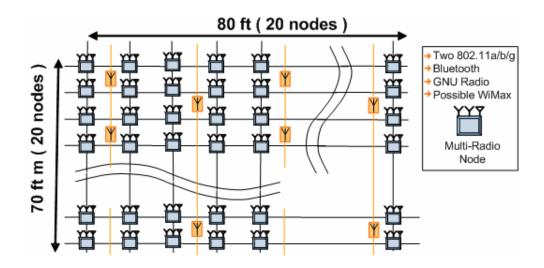
Fig. 8 ORBIT multi-radio grid testbed
