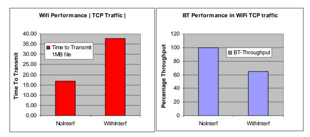
Fig 11 (a) Time to transmit (in seconds) a 1MB file between WiFi pairs (b) Bluetooth throughput with a background WiFi TCP 1MB file transfer operation.
