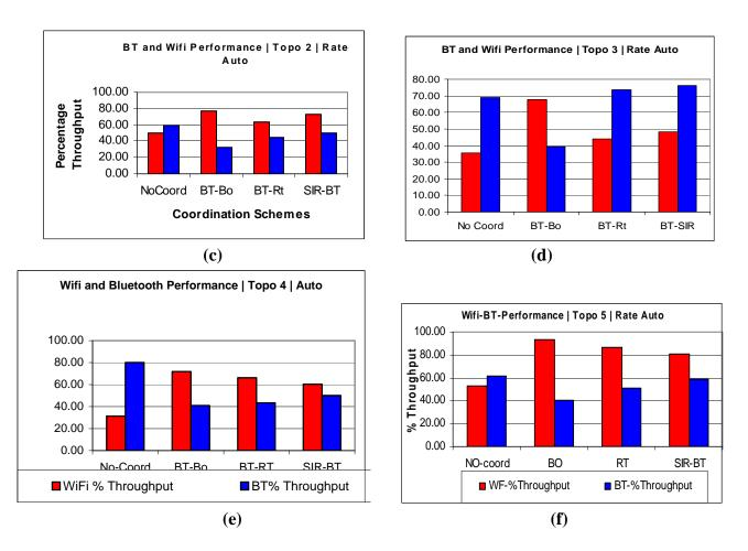
Figure 13 Results for WiFi-BT throughput vs. Coordination Scheme, Fig 13(c-f) correspond to Topologies 9(c-f)
