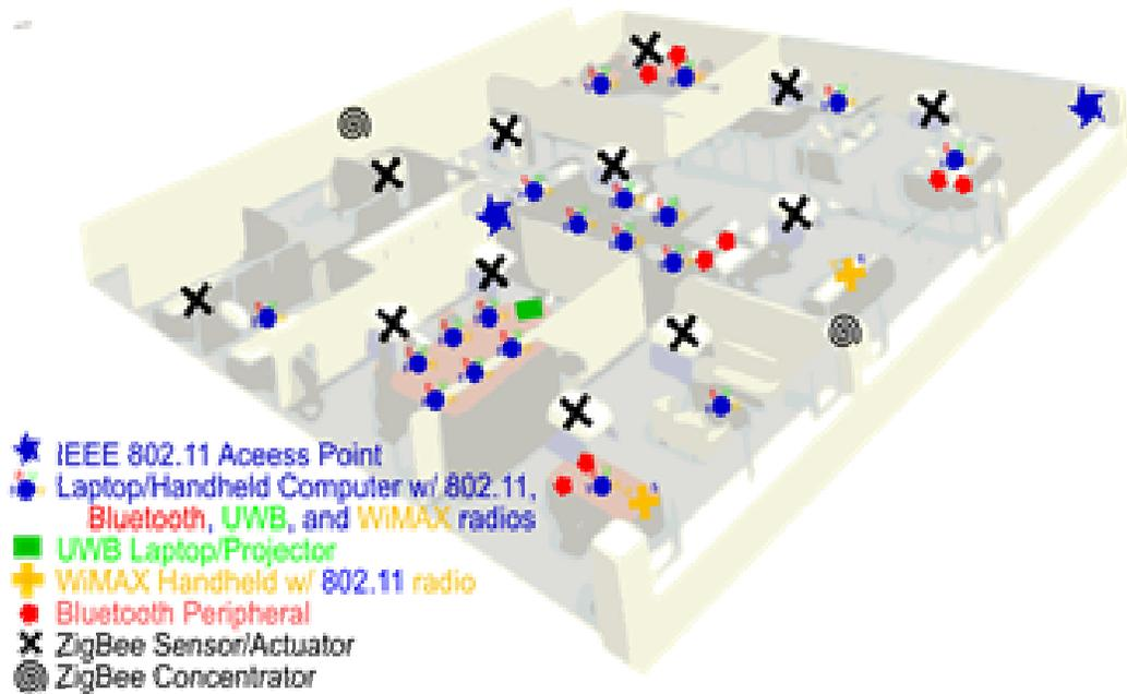
**Fig. 1 SOHO scenario for multi-radio co-existence.**
