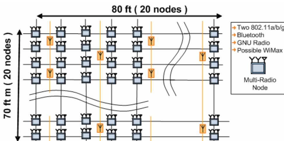
**Fig. 8 ORBIT multi-radio grid testbed**
