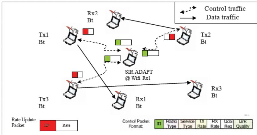
**Fig. 6 SIR-BT Rate Adaptation for Wifi/BT Coexistence.**
