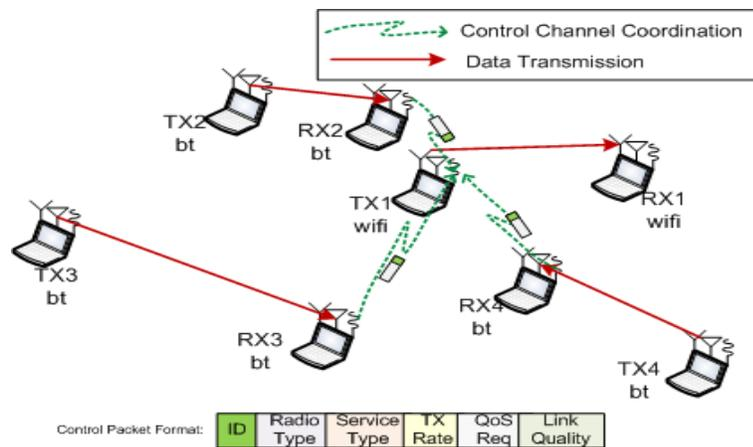
**Fig 4 CSCC protocol in an IEEE 802.11g and Bluetooth coexistence scenario.**
