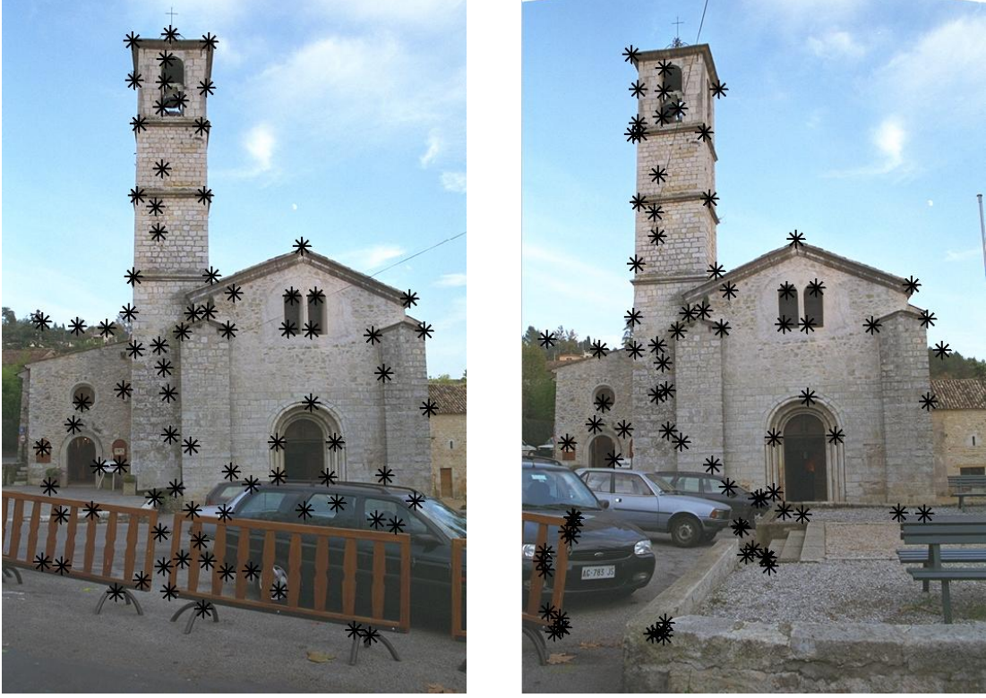
Figure 4.12: Fundamental matrix estimation for the Valbonne sequence. Both images are shown along with the 85 point matches (inliers and outliers).
