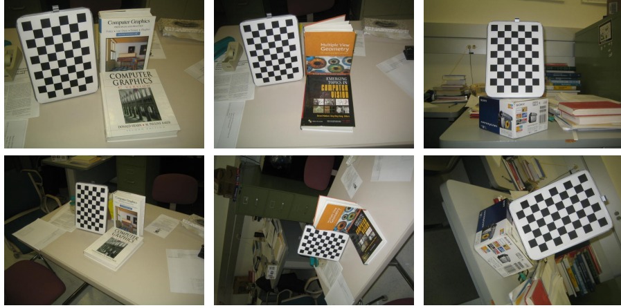
Figure 3.3: Camera Pose Segmentation . Images used to reconstruct 3D point clouds using the OpenCV implementation of the calibration technique of [142]
