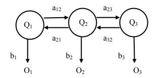
**Figure 12:** A graphical depiction of an HMM with states  $Q=Q_1, Q_2, ..., Q_T$ , observations  $O=O_1, O_2, O_3, ..., O_T$ , transition probability matrix  $A=\{a_{ij}\}$ , and emission probability matrix  $B=\{b(o|S_j)\}$ .
