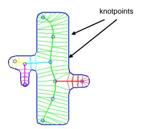
**Figure 10:** Example shape with its skeleton, ribs, and knotpoints, which are used as the terminals in the context free grammar model.
