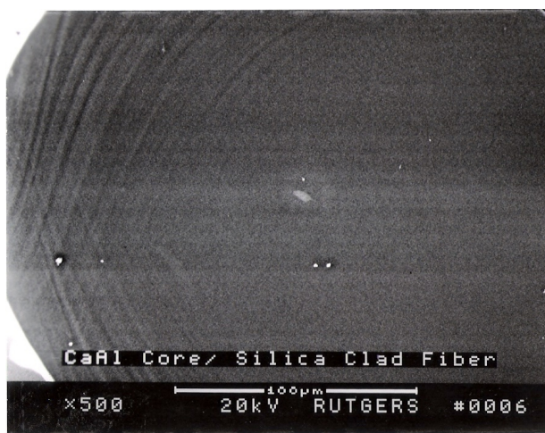
Figure IV.10 - SEM Photomicrograph of 8 \mu\text{m} /250 \mu\text{m} CAG/Silica Fiber
