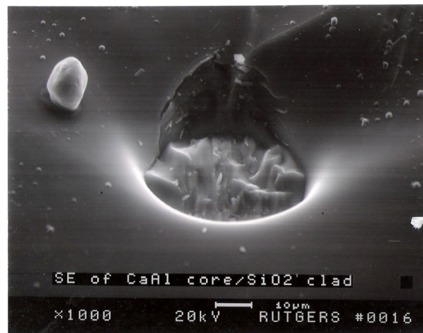
Figure IV.9 - SEM Photomicrograph of CAG Core/Silica Clad Fiber Core Region - Close up
