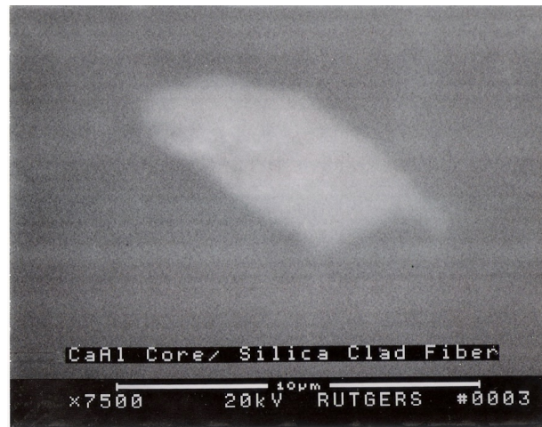
Figure IV.11 - SEM Photomicrograph of 8\text{ }\mu\text{m} / 250\text{ }\mu\text{m} CAG/Silica Fiber Core Region Close up
