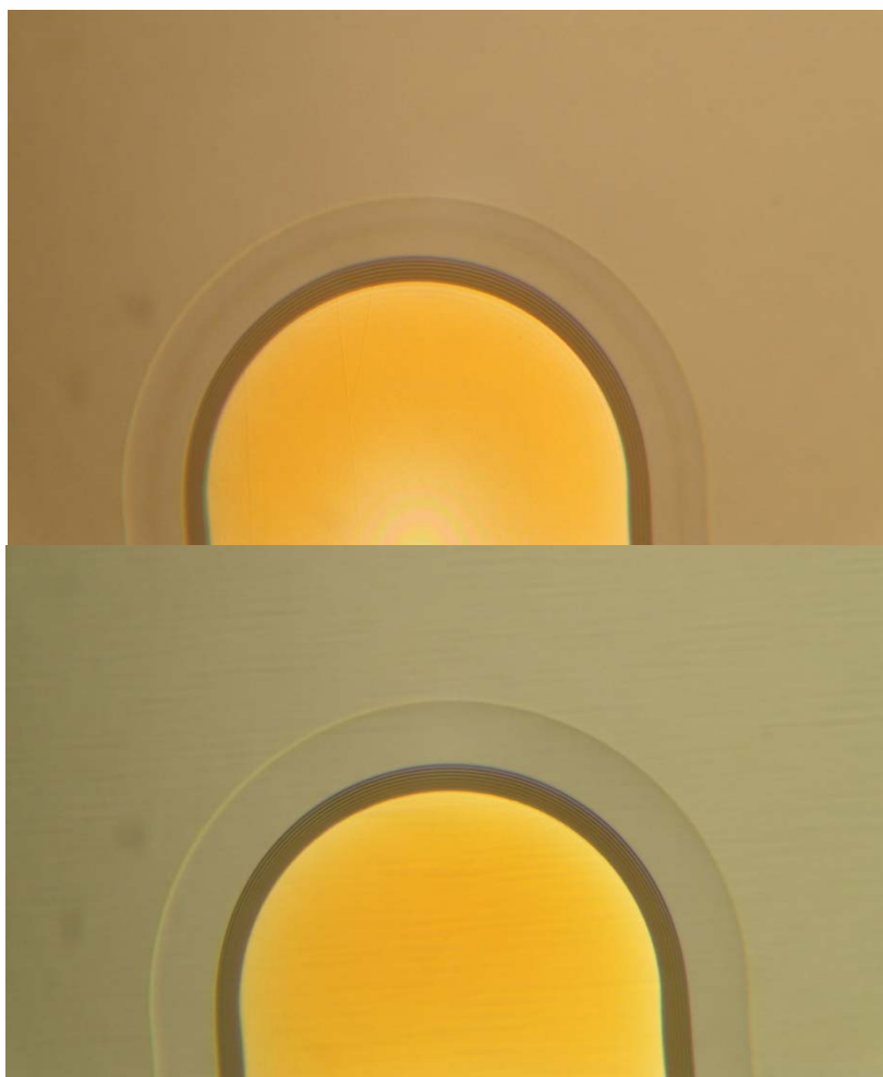
Fig. 3-10 SiC bevel surfaces with \text{CF}_4 flow rate of 60sccm and 5sccm, respectively. The top one shows a rough surface etched at 60 sccm. The bottom one shows a smooth surface etched at 5 sccm.
