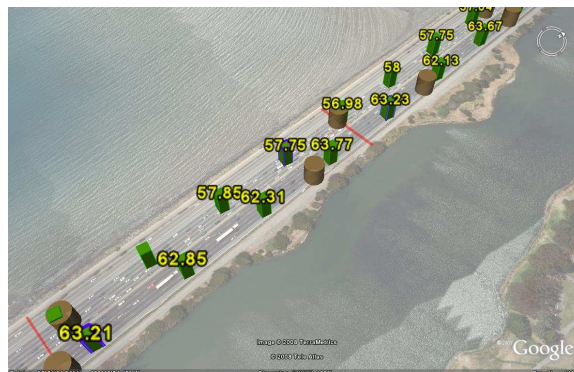
Figure 8.9: Satellite image of the first experiment site I-80 near Berkeley, CA. The red lines represent the locations of the VTLs, the blue squares show the speed recorded by the VTL, the green squares represent the position and speed stored in the phone log. The brown circles represent the readings from the vehicle speedometer.
