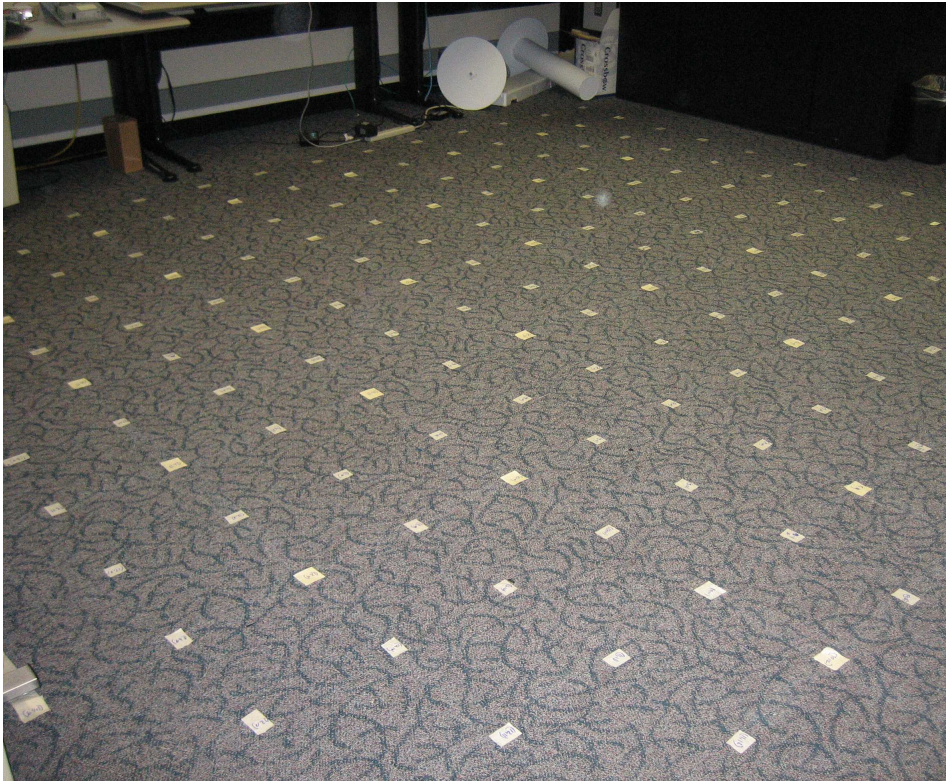
Figure 5.13: Photograph of deployment area showing that all motes are in line-of-sight with no obstructions in between.
