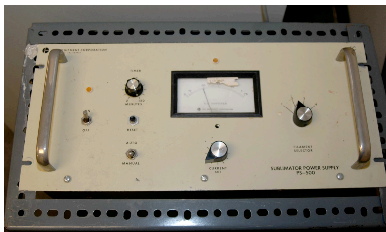
Figure 2.4. Low-current sublimation power supply used to sublimate organic materials
