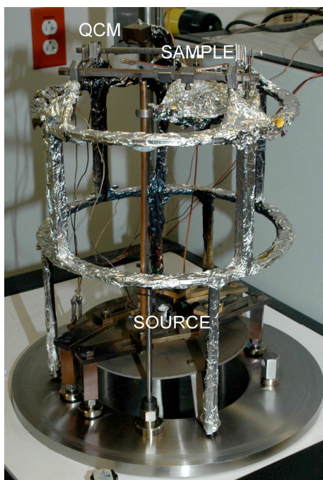
Figure 2.3. Scaffolding elevates the sample above the source for line-of-sight deposition of sublimated and evaporated materials.
