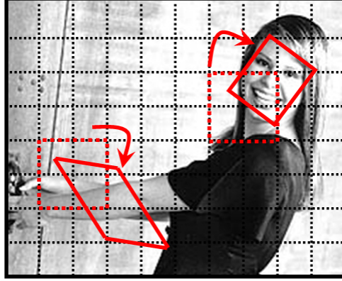
Figure 5.7: The trackers are initialized at sparse regular grid (dashed boxes). Final locations (solid boxes) are evaluated with face detector and the nonface regions are rejected.
