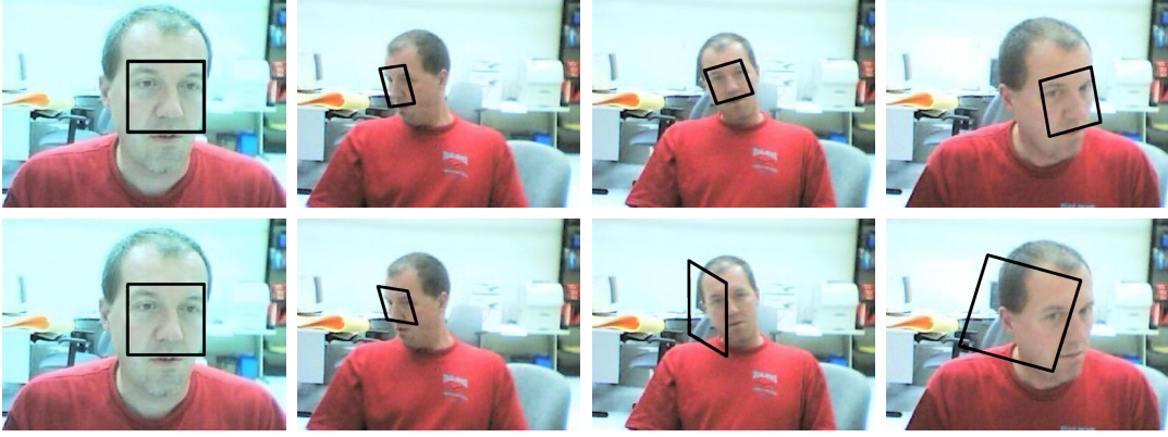
Figure 5.10: The effect of model update. The first row is with update. The second row is without update. The target has severe appearance variations due to illumination and pose change throughout the sequence. The sequence contains 324 frames.
