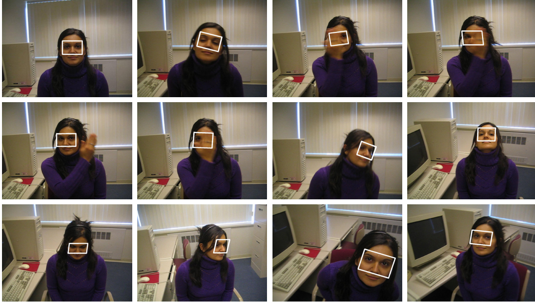
Figure 5.12: Affine tracking of a face. The target has large on-plane and off-plane rotations, translations, scale, illumination and appearance changes and occlusions. The sequence contains 425 frames.
