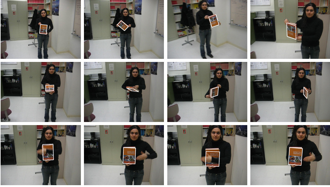
Figure 5.11: Affine tracking of a book. The target has large on-plane and off-plane rotations, translations, scale changes and occlusions. The sequence contains 739 frames.
