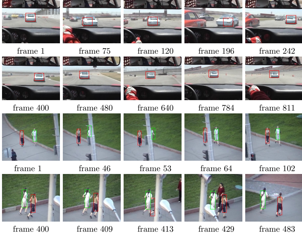
Figure 3.8: Tracking results using for moving camera sequences. Size changes (frames 75, 196, 242, 881) in Race sequence and severe occlusions (frames 53, 64, 409, 413) in Jogging sequence are accurately detected.
