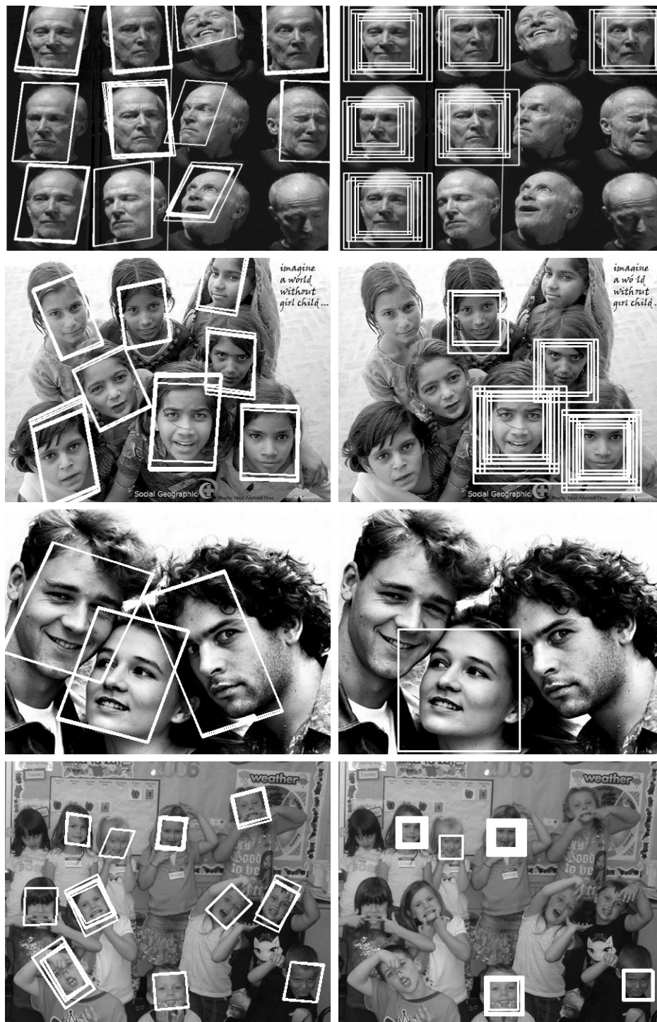
Figure 5.16: Face detection examples using the proposed method ( first column ) and the original VJ detector with a dense scan ( second column ). The original VJ detector is very sensitive to pose changes.
