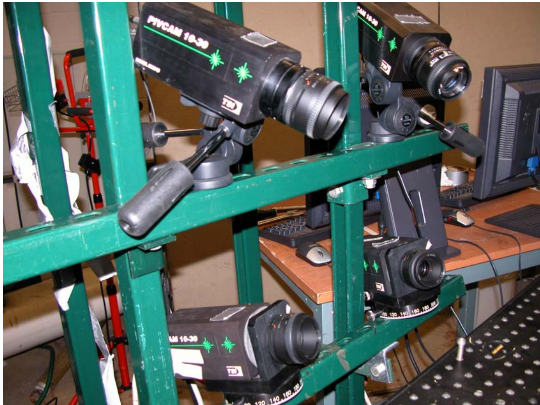
Figure 3.2. Photograph showing the rectangular arrangement of the four cameras. The four cameras were rotated and tilted to focus on the same region in the measurement tank (not shown)
