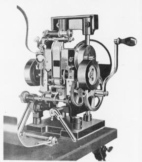
This cut shows the mechanism of our absolute flickerless New Model. Observe the mechanically correct construction; note the two fly-wheels, one on each side of the frame, thus assuring perfect motion, see the spiral gears; look especially at the POSITIVE Rewinding Attachment which can never go wrong and which in itself is a marvel of perfection.
