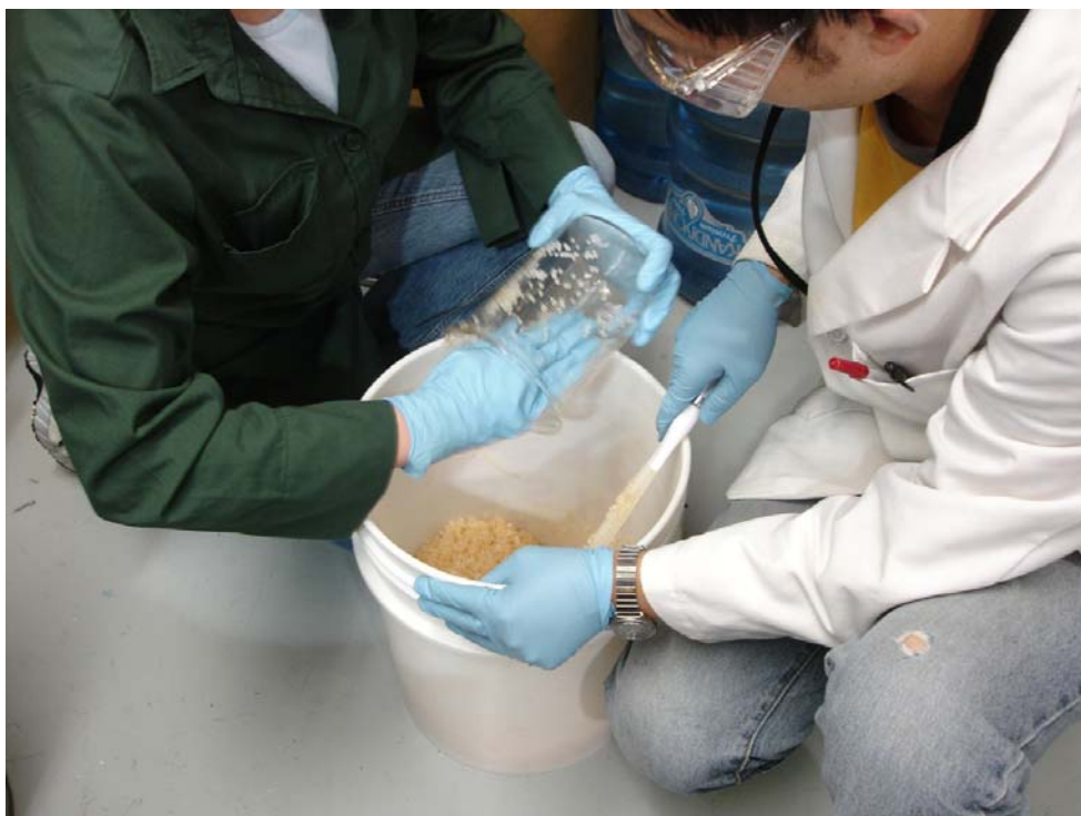
Figure 27- Mixed tocopherols being manually plated onto 10% of the polymer resin.
