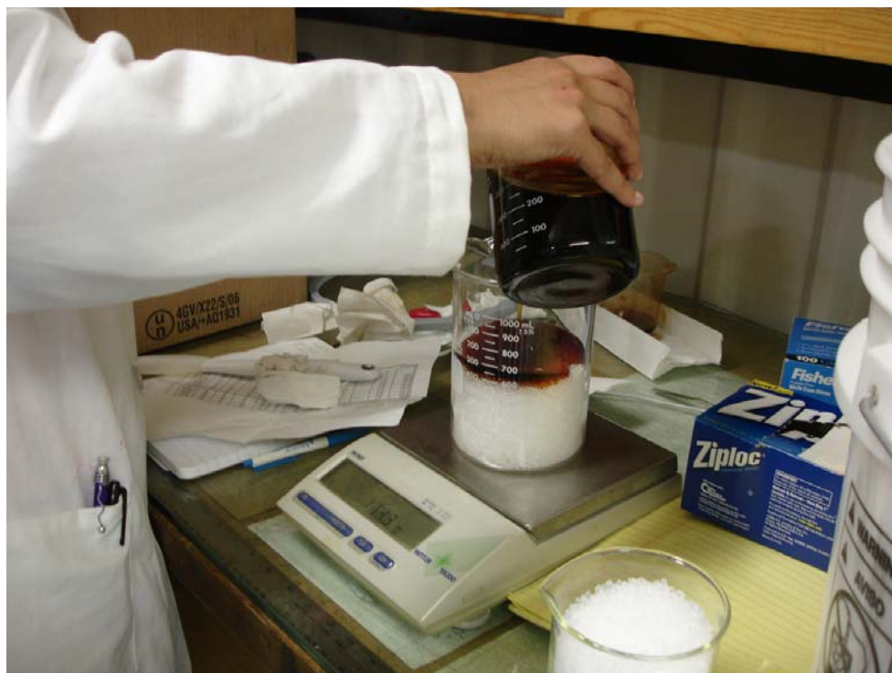
Figure 26 – Mixed tocopherols being weighed onto a small amount of polymer resin.
