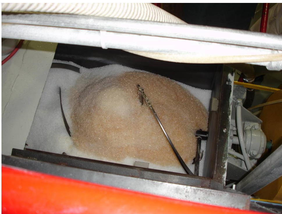
Figure 28 - Ribbon mixer used to blend tocopherol coated resin and remaining polymer resin.
