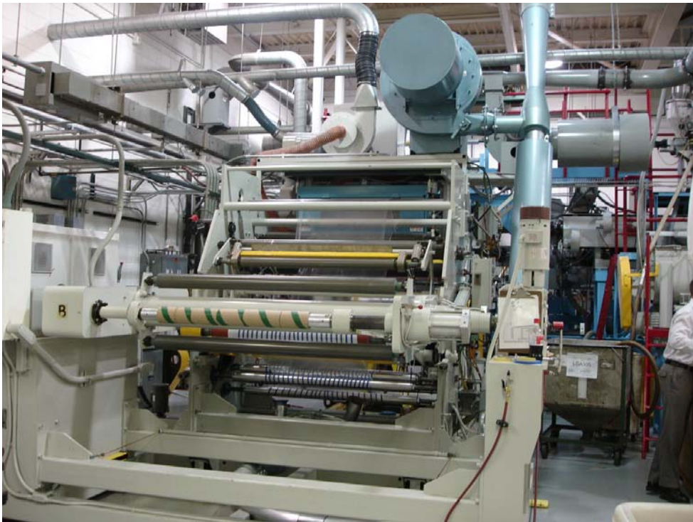
Figure 25 - Parkinson winder used in film production.
