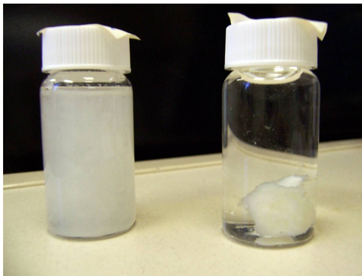
Figure 3. Control (left) and mineralized DBM (right) in DI water following intense agitation, demonstrating increased fiber cohesivity afforded by the mineral phase.
