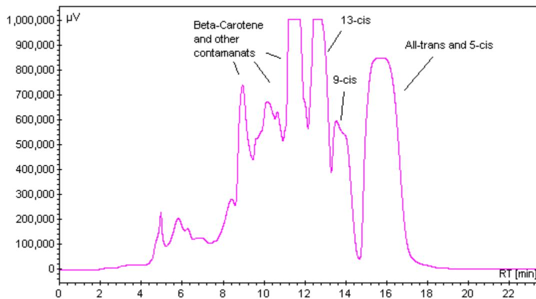
Figure 2. A typical chromatogram of isomerized lycopene using a Develisil RP-Aqueous column with the analytical HPLC method.
