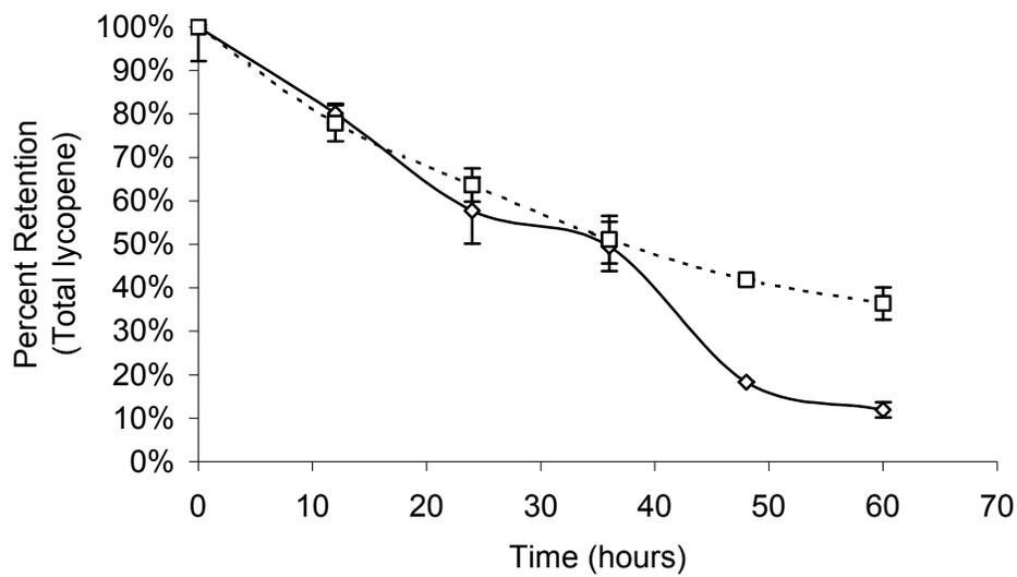
Figure 8. Percentage of cis isomers (of the total lycopene) during storage at 35°C; (—) cis lycopene in MCT, (----) cis lycopene in MCT encapsulated in gum acacia (1.25% MCT dry weight).
