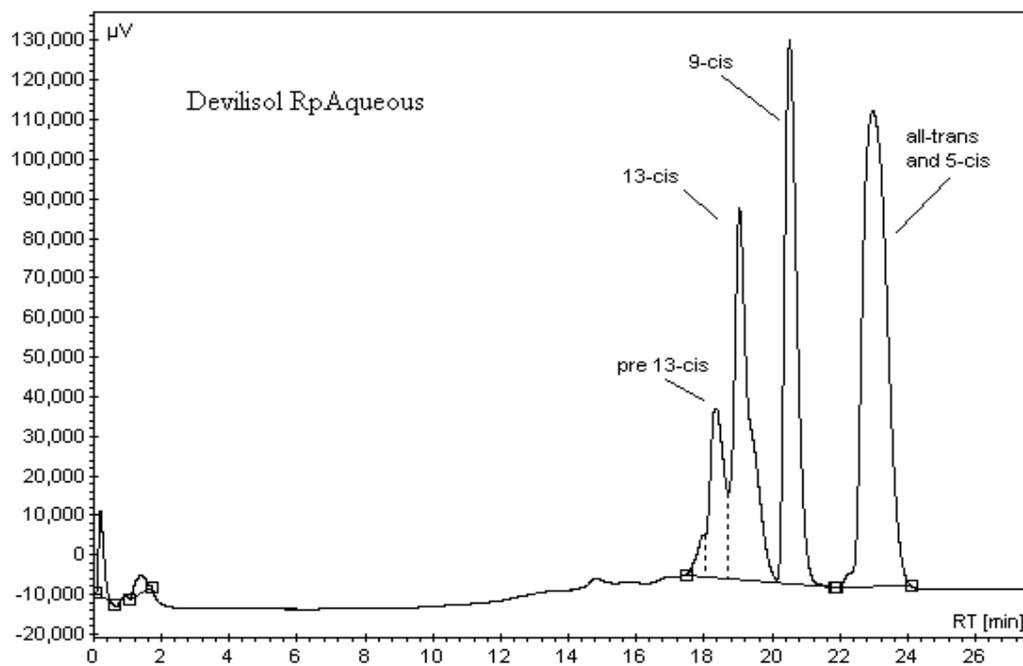
Figure 3. A typical chromatogram of isomerized lycopene using a YMC carotenoid column with the analytical HPLC method.
