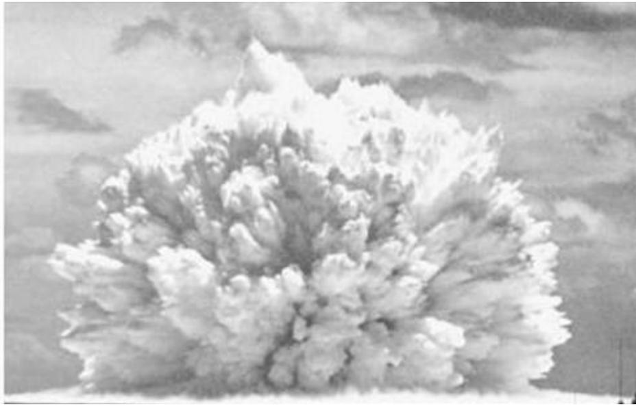
Fig. 2.13. Hemispherical blast waves for ground-level explosion (courtesy Reuters)
