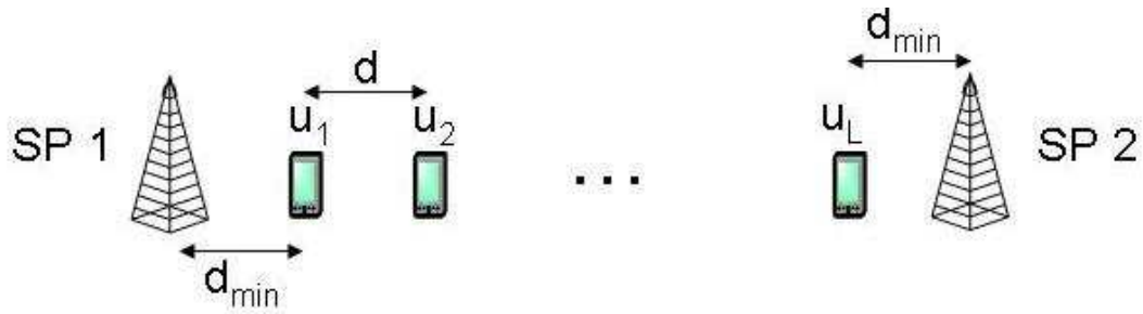
Figure 6.2: The network topology for two SPs and L users. For a single SP, assume either SP 1 or SP 2 is present
