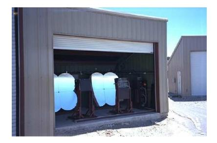
Figure 2.5: HiRes-II Mirror Building. Showing Ring 1 (right) and Ring 2 (left), cluster boxes and electronics rack.
