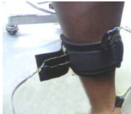
Figure 26 This figure shows the FMG Cuff placed on the lower portion of the calf muscle. Wires can be seen coming from the four FSRs placed within the cuff.
