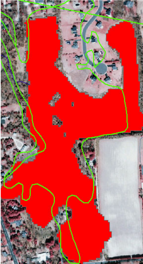
Figure 173: FEMA Q3 data (green line) overlaying floodplain (red polygon) for Albers Pond
