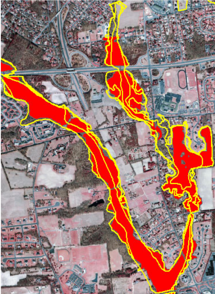
Figure 145: Modeled and DFIRM 100-year floodplain for Wreck Pond Brook (Hwy 138 to Allaire Rd) and Albers Pond Creek
