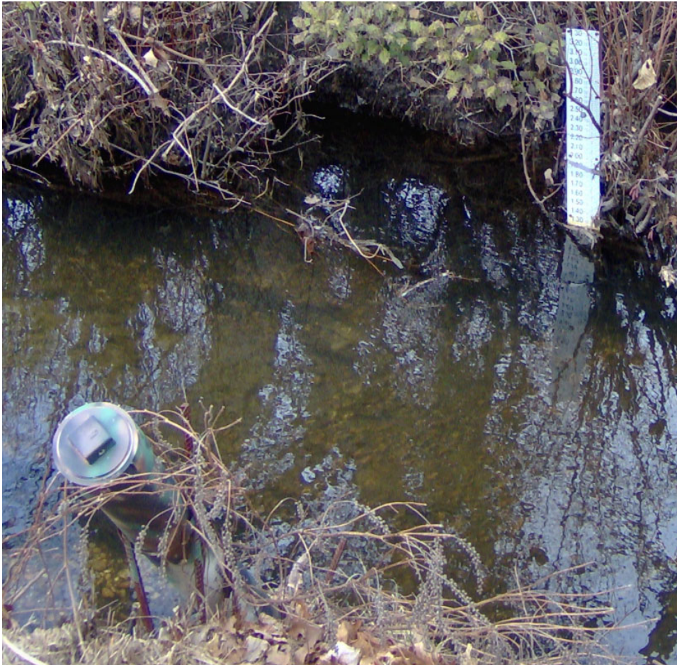
Figure 101: Staff gage and miniTroll instrument housed inside PVC pipe anchored in a concrete block
