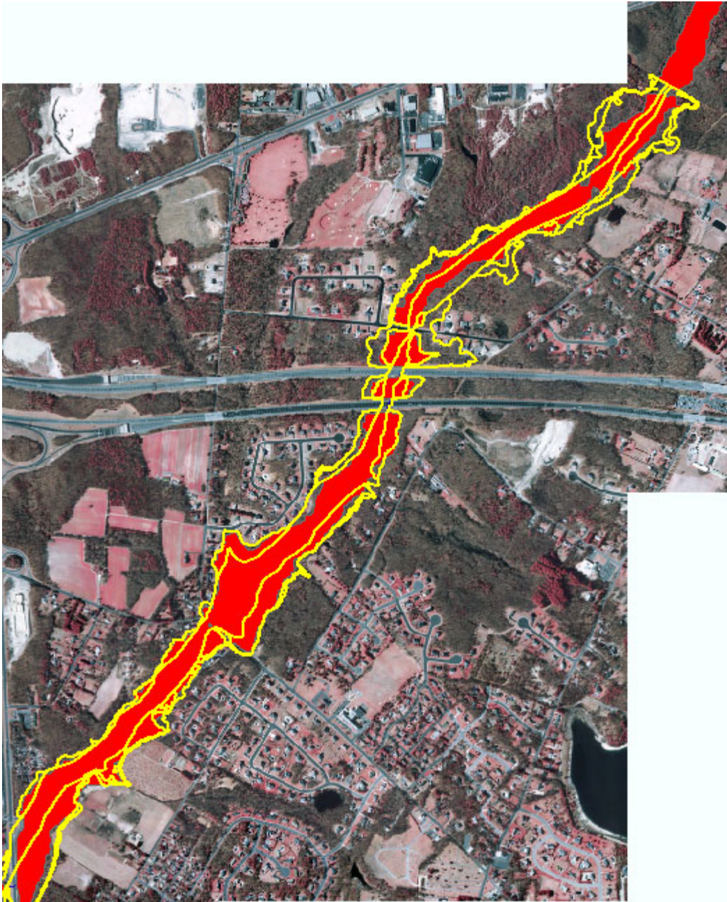
Figure 144: Modeled and DFIRM 100-year floodplain for Wreck Pond Brook (up to Hwy 138)
