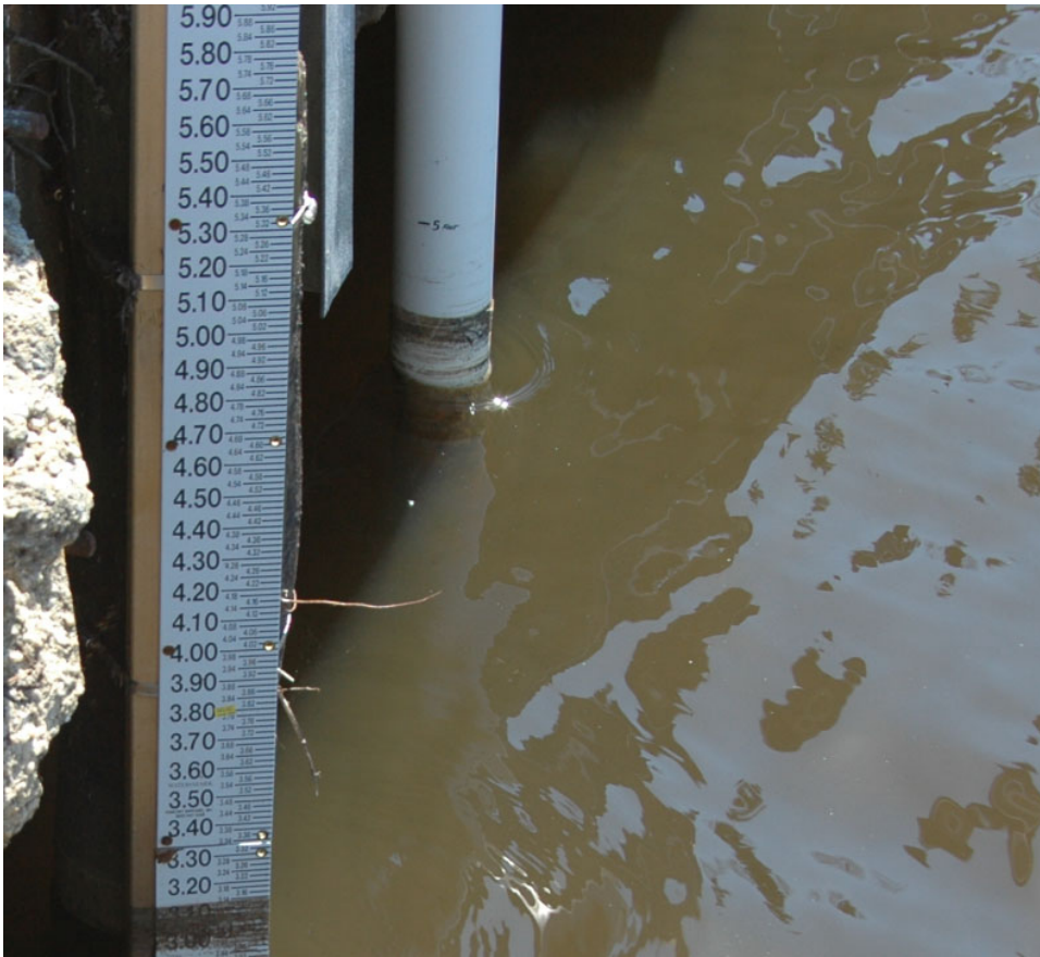
Figure 102: Staff gage and miniTroll instrument housed inside PVC pipe and anchored to a culvert
