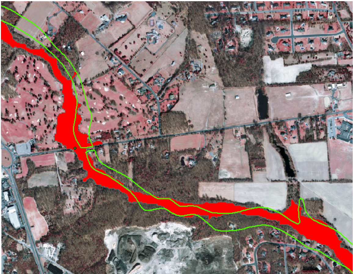
Figure 172: FEMA Q3 data (green line) overlaying floodplain delineated (red polygon) - location on Hannabrand Brook
