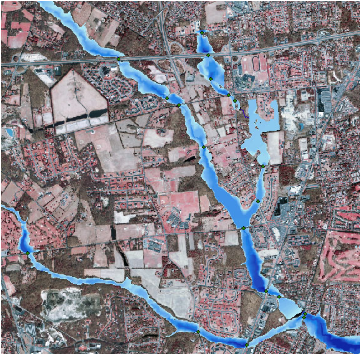
Figure 142: Water depth grid overlaying Aerial photos
