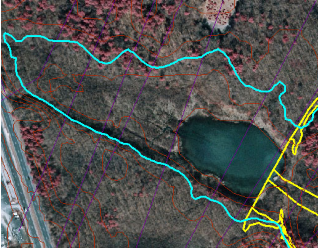
Figure 181: DFIRM line for 1% chance and storage analysis at Keller's pond
