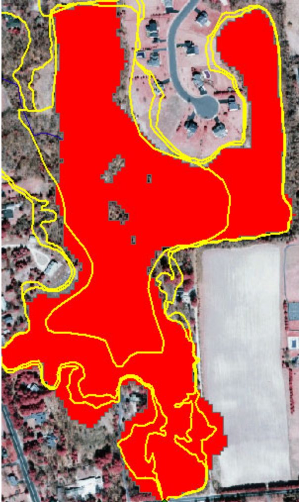
Figure 175: DFIRM (yellow line) overlaying modeled floodplain (red polygon) for Albers Pond
