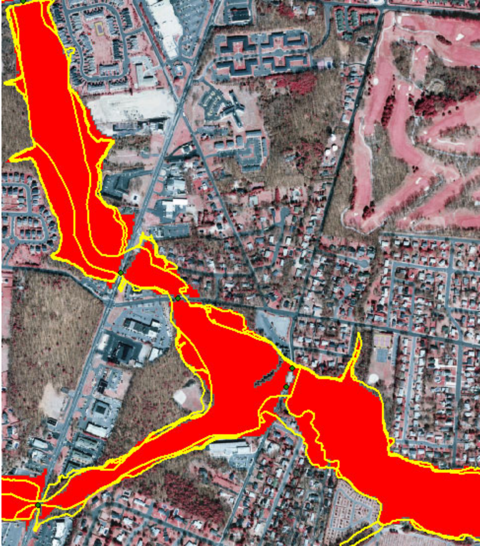
Figure 146: Modeled and DFIRM 100-year floodplain for Wreck Pond Brook (Allaire Rd to just downstream of Old Mill Pond)
