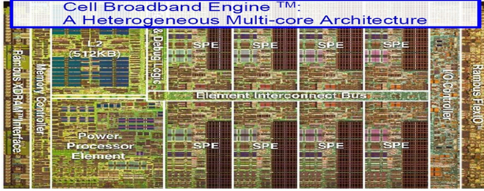
Figure 6.8: The multi-core architecture of the IBM Cell/B.E.
