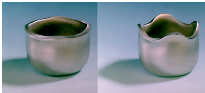
Figure 1.2: Cup formed by deep-drawing a rolled sheet. The 'ears' are evidence of texture-caused anisotropy. [aluminium.matter.org.uk]
