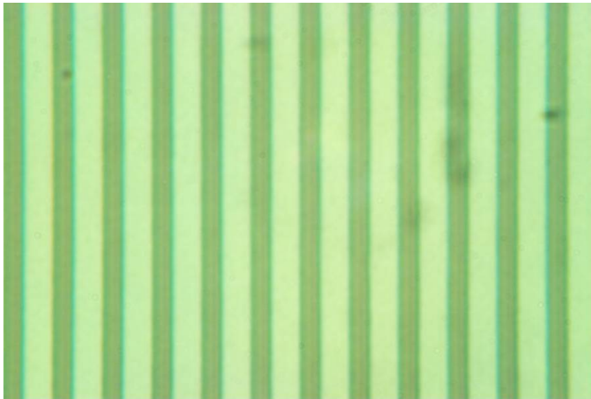
Figure 5.5. Optical microphotograph of AlTi pattern for ICP etching of mesas. The periodicity of the structure is 5.2μm.
