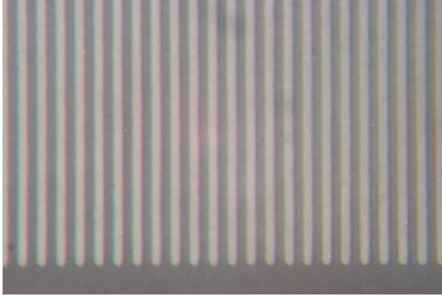
Figure 4.7. Optical micrograph of AlTi pattern for ICP etching of mesas. The periodicity of the structure is 2.5\mu\text{m} .
