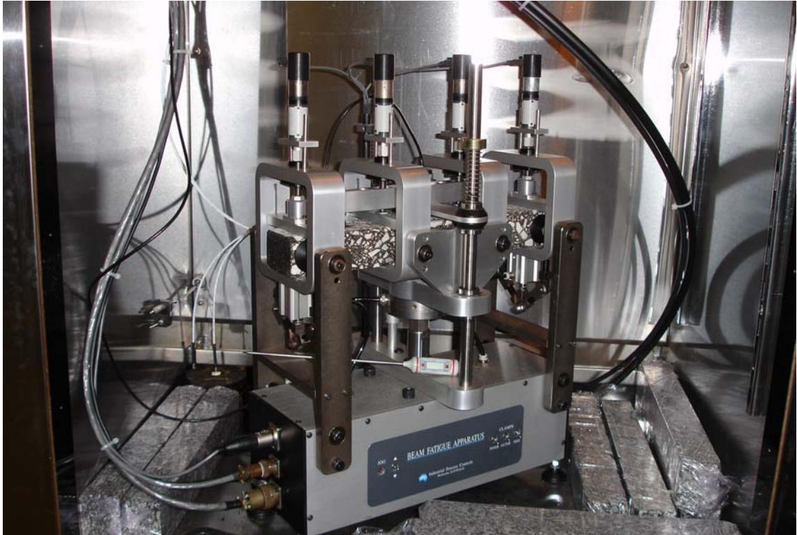
Figure 4.6 – Flexural Beam Fatigue Test Device
