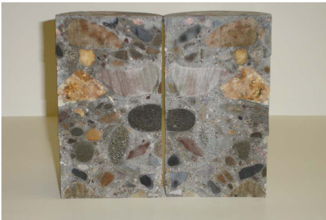
Figure 5.23 – Cross Sectional View of PCC Core Taken from Rt 202S in New Jersey
