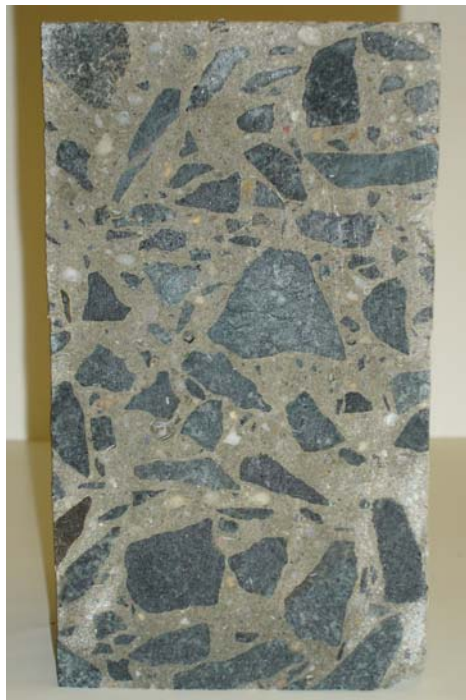
Figure 5.32 – Photo of PCC Core Taken from Interstate 495 in Massachusetts
