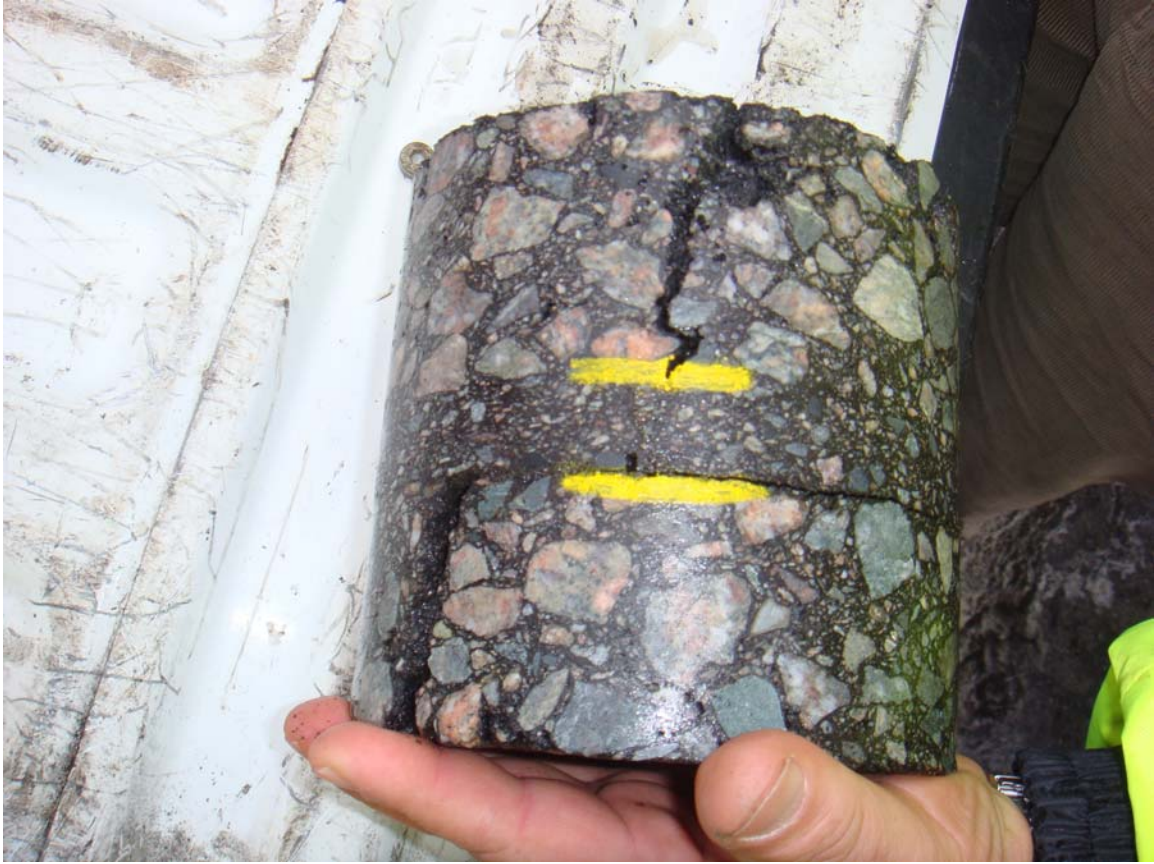
Figure 7.19 – Photo of Core Taken Through Surface Crack on I495 in Massachusetts
