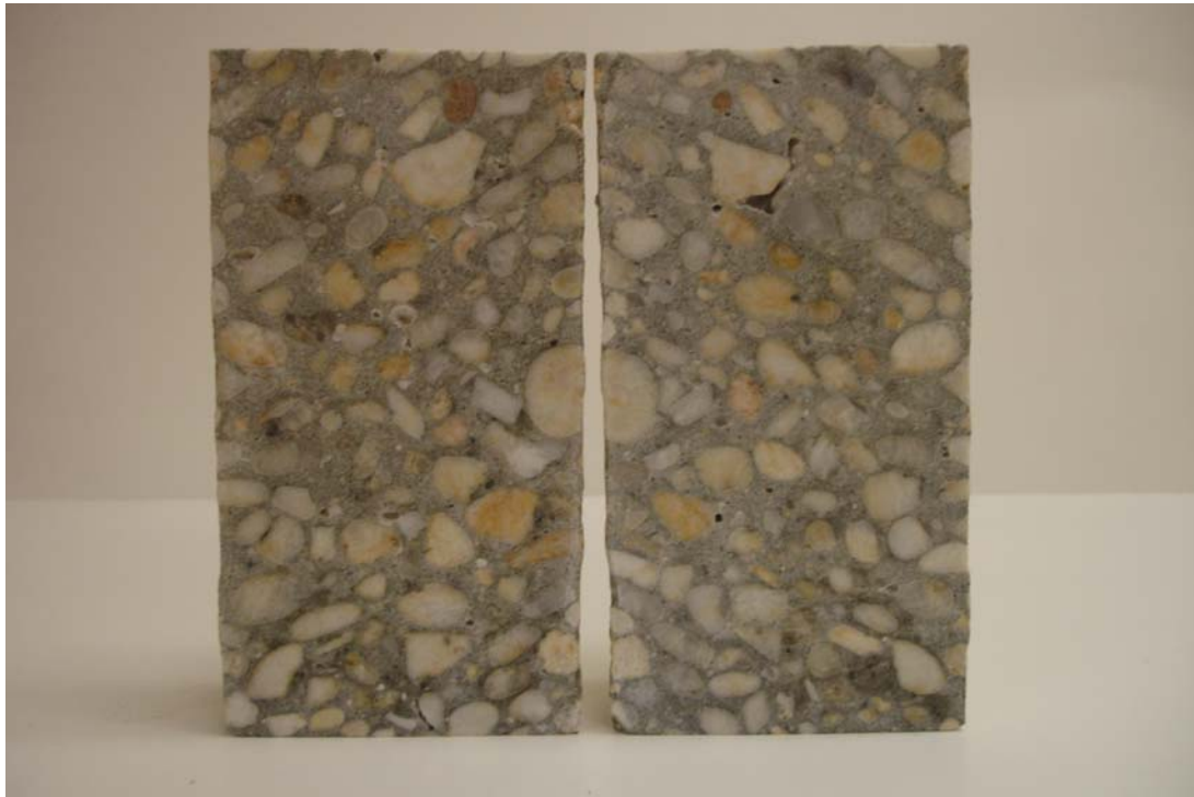
Figure 5.11 – Cross Sectional View of PCC Core Taken from Rt 34N in New Jersey
