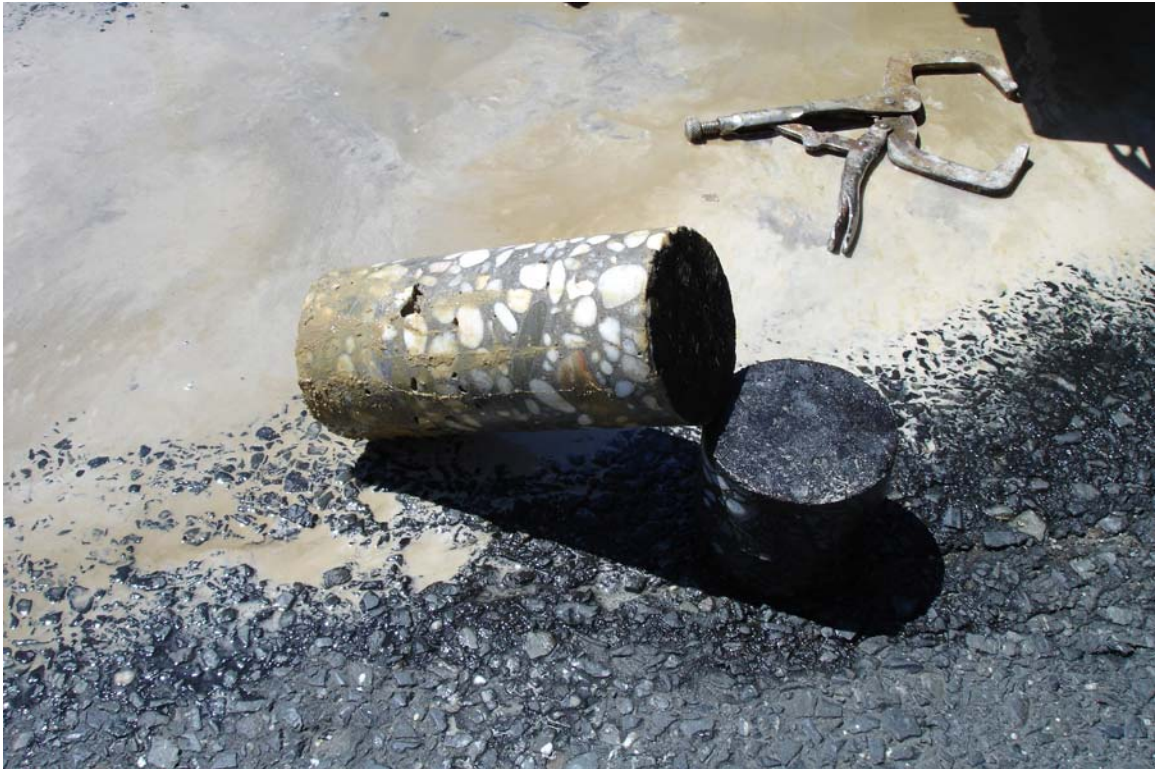
Figure 4.4 – Extracted Portland Cement Concrete Core from Pre-Overlaid Pavement
