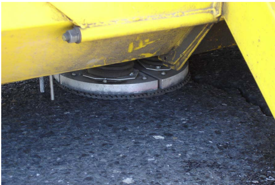
Figure 4.3 – Falling Weight Deflectometer (FWD) Testing at the PCC Joint
