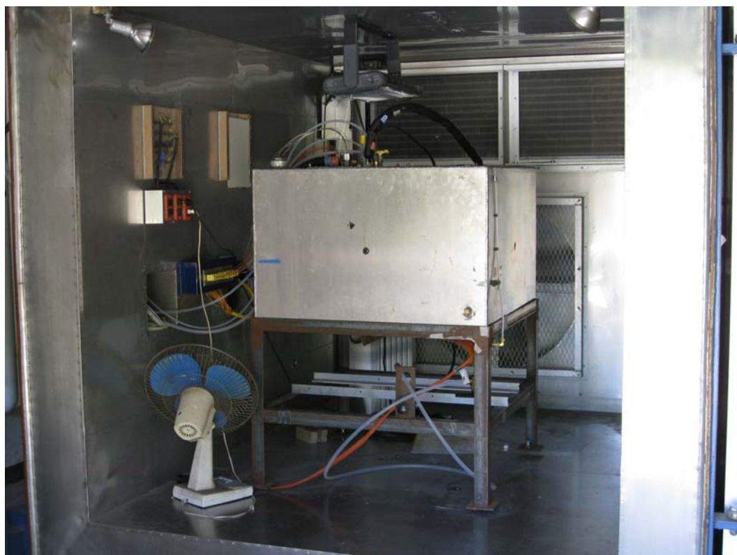
Figure 3.1 Fuel tank placed in the altitude chamber
