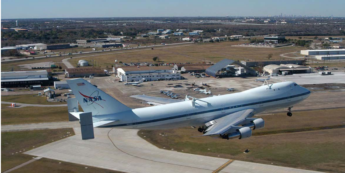
Figure 5.14 NASA 747 SCA used for gathering flight test data. 9
